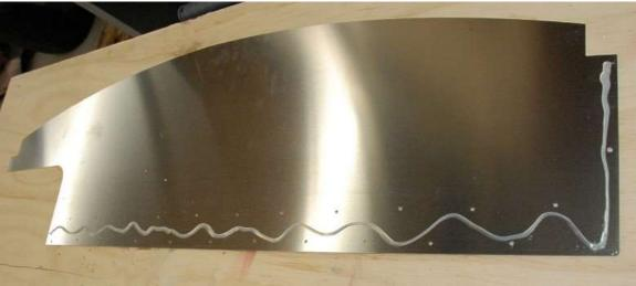
Mark the firewall and drill for riveting.
