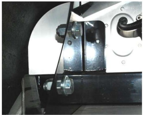
Slide the windshield into position and bolt in place using the windshield mounting hardware. Snug the bolts up so that the angle can get set.
