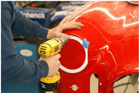
Drill the two smaller corner holes with a  $\frac{1}{4}$ " drill bit to mark their location. Follow this with a  $\frac{3}{8}$ " drill bit.
