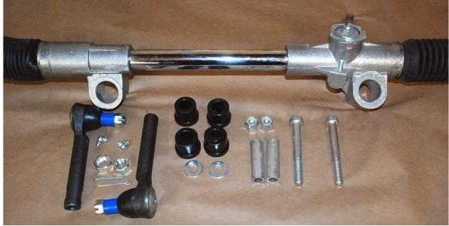
Unpack the manual steering rack and the mounting assembly.
