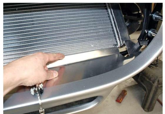
Position the radiator floor aluminum so that it goes under the body lip and goes across to the bottom of the radiator. Clamp the floor piece to the nose.
