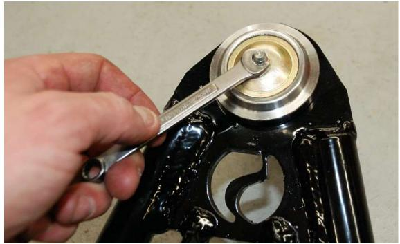
Screw the grease fittings into the arms using a  $\frac{5}{16}$  wrench.
