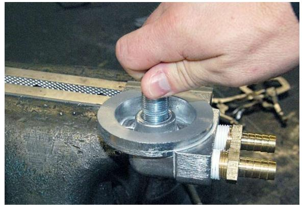
Thread the short end of the threaded nipple into the relocator.
