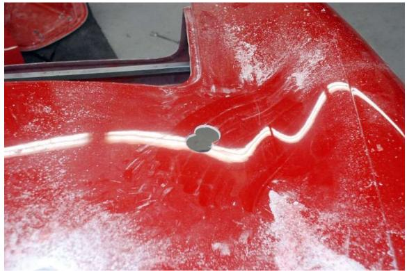
The rear of the hole is then finished using the whole saw vertically.
