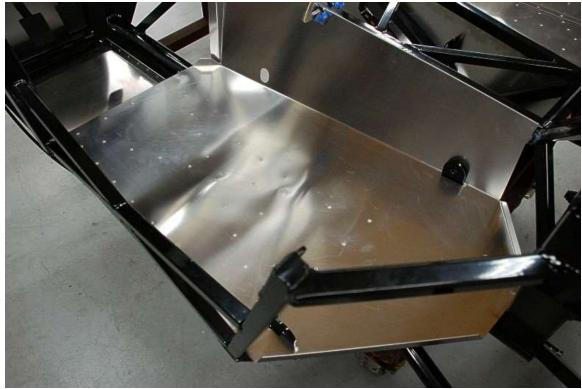
Silicone, drill, and install the driver side floor.
