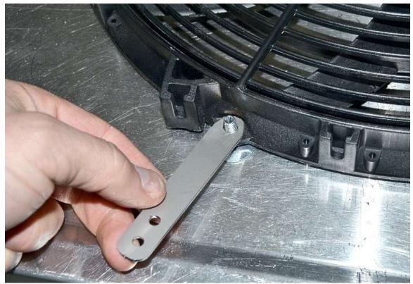
Put the fan mounting strap on top of the fan using the larger single hole at the end.
