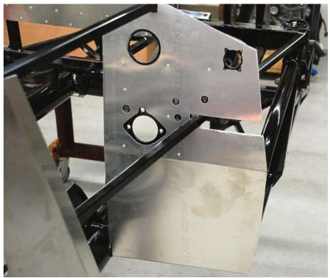
Mark, drill, and rivet in place the left side footbox front panel, do not silicone or rivet the right lower section that attaches to the <sup>3</sup>/<sub>4</sub>" vertical tube in order to allow the inside wall to slip underneath.
