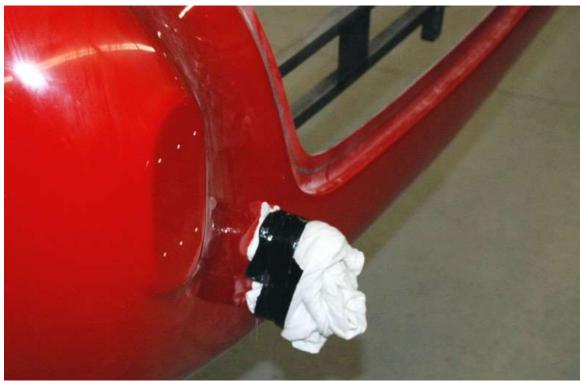
Even with the quick jacks removed, it is still a good idea to wrap the bolts with some rags and duct-tape to save yourself from painful cuts or bruises.
