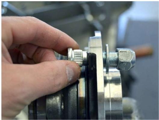
Insert one of the included wheel studs into the hub from the back and use a washer and lug nut on the front side.
