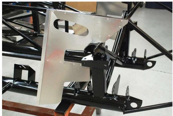
Rivet the panel in place using 1/8" short rivets, then remove the screws and replace them with rivets. Repeat for the other side.
