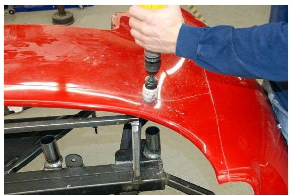
The roll bar holes are marked on the body and need to be cut out using a  $1^{3}$ /4" holes saw. The front two holes are cut centering the saw in the marked circle and drilling vertically to match the angle the bar comes through the body.
