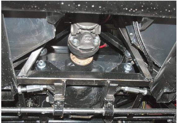
Insert the driveshaft into the transmission, bolt the rear flange to the driveshaft adapter and torque the bolts to **95Nm** (**70 lb-ft**).
