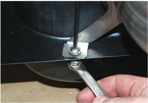
Use the <sup>1</sup>/<sub>4</sub>" bolt and locknut to attach the retainer to the tank.
