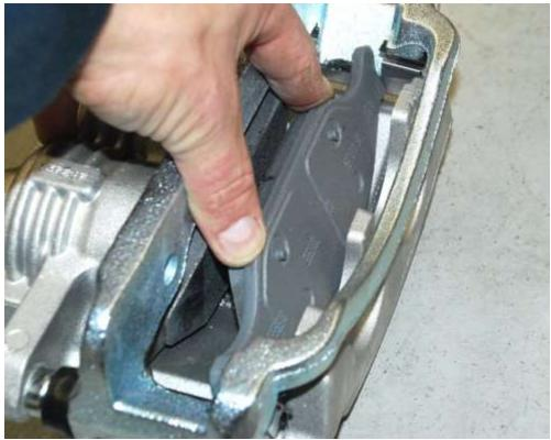
Install the brake pads in the Caliper.
