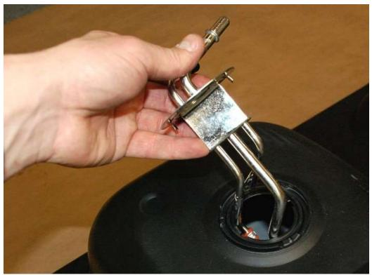
Slide the pickup down into the tank; you will have to rotate as you go to get the tubes into the sump and line up the tabs on the pick-up and slots on the tank. You can see this looking through the filler neck hole.
