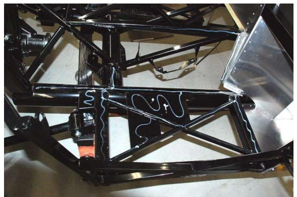
Silicone the chassis where the aluminum floor will touch. The main chassis rails are not riveted to but still need a bead of silicone run along the tops. The top edge of the tunnel is not riveted yet but gets silicone as well.
