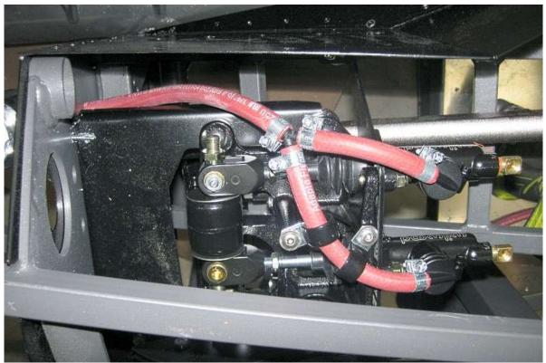
Connect and split the hose to the two master cylinders using the Y provided. Make sure that the line cannot get in the way of moving parts, especially the brake pedal!
