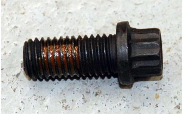
The driveshaft bolts are in the box with the driveshaft and should have thread locker on them already. If thread locker is not there, put a small bead on each bolt.
