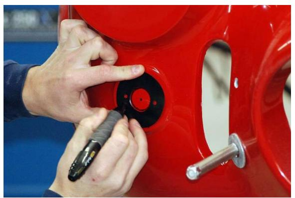
Remove the gasket from the turn signal box and use it to center and trace the mounting holes and large center hole for the turn signal.
