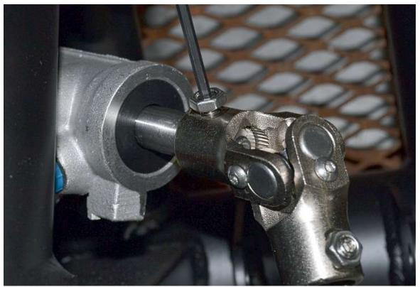
Push the shaft into the steering joint so that the set screw will go into the recessed area on the input shaft then tighten the set screw and jam nut using a  $\frac{5}{32}$ " Hex key and  $\frac{1}{2}$ " wrench.
