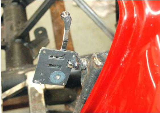
Latch the door latch onto the striker and close the door. Adjust the striker if needed to fit the latch to the door cut out. You can also use the door latch spacers to help with this alignment.
