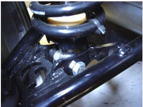
Run zip ties through the holes in the spring hat and around the spring to prevent the spring from becoming unseated.
