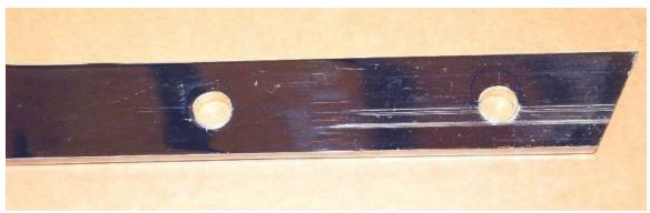
At the marks made on the sidebar, measure and mark the center of the sidebar to give the correct angle adjustment on the windshield. Drill the holes with a  $\frac{1}{2}$ " bit.
