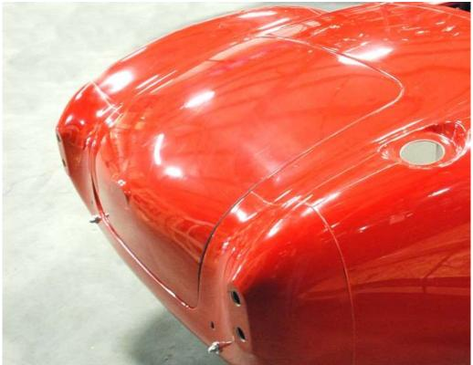
Close the trunk and wiggle it into position then open and tighten the bolts. This may take a little adjustment to get the trunk to sit down right. You can also use some of the rubber bumpers from the hood opening as a temporary means of holding the surfaces level.
