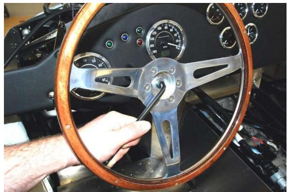
Bolt the steering wheel assembly to the steering shaft. Use thread-locker on this bolt.
