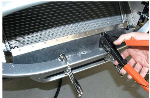
Silicone and rivet the aluminum to the nose lip using three 3/16" rivets.
