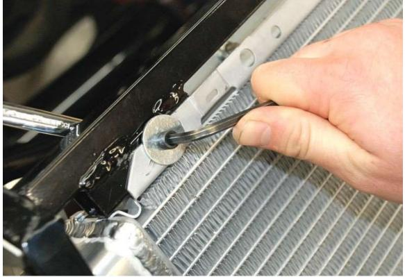
Mount the radiator top to the flange with the hardware provided. The bottom stays zip tied for now.
