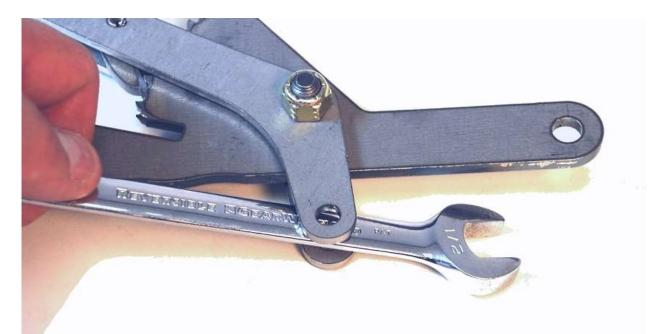
Use a wrench to spread the ears of the ratchet to handle mounts so that the rod end can just slide between them.
