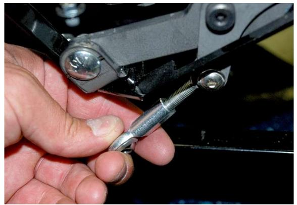
Release the brake and if necessary, remove the <sup>1</sup>/<sub>4</sub>" clevis bolt and readjust the rod end so that the cable is tight.
