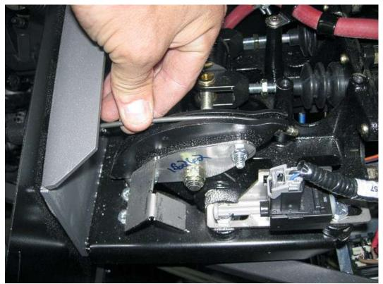
Slide the clutch cable boss through the firewall spacer and loop the cable over the quadrant.
