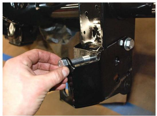
Temporarily put the lower shock bolt through the traction lock bracket and stock shock hole on the axle.
