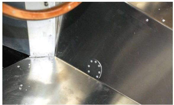
Silicone and install the tunnel plug patch panel.
