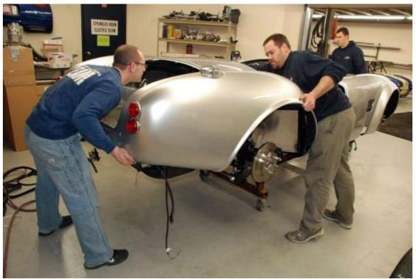
Fit the body back on the chassis. Be very careful with the sides and slowly work it down into position. Pull the sides out around the chassis and make sure the body covers the rear cockpit wall and top of the dash without pulling the material off either.
