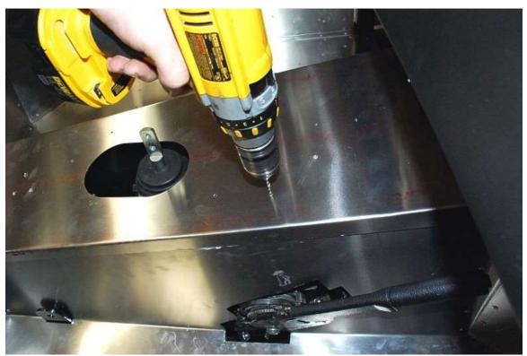
Silicone and install the transmission tunnel top.
