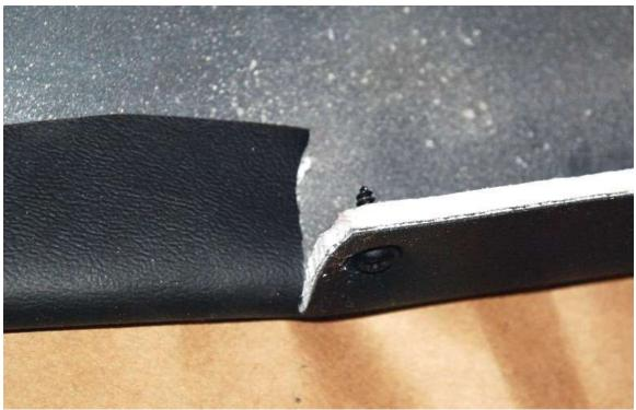
If you are having trouble getting the pad to stick on the bottom of the dash you can screw the corners down using some of the trim screws provided with the dash hardware.
