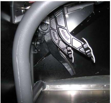
Adjust the clutch pedal stop and master cylinder threaded shafts so that the pedal height is comfortable. In general, the clutch pedal is about 2" higher than the brake pedal and the brake pedal is higher than the accelerator pedal so that when the brakes are pressed the brake pedal is even with the accelerator pedal.
