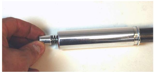
Screw the button onto the end of the anchor bolt.
