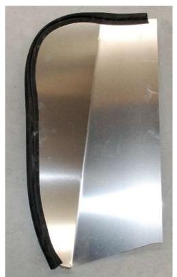
Put some of the press-on bulb seal around the outside edge of the aluminum front splash guards (they look like large elephant ears) where they will contact the body.
