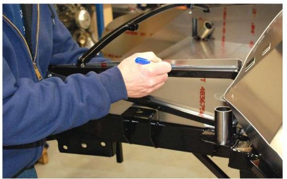
Using a marker outline the underside of each panel where it contacts the chassis. This is done to locate where to drill rivet holes when the panels are permanently mounted later on.
