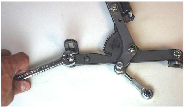
Attach the mount brackets to the fixed gear using a  $\frac{1}{2}$ " wrench. Leave the locknut slightly loose so positioning can be done on the frame later.
