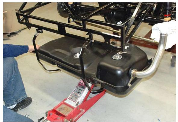
Using a jack, raise the tank up into place on the chassis. Make sure the plastic cover is in position below the tank.
