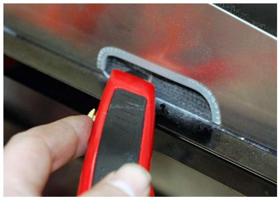
Cut the carpet with a single slit to allow the harness to pass through.
