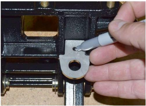
Place the switch mount between the brake pedal mount tabs on the side closest to the brake pedal pivot holes and drill a  $\frac{3}{16}$  hole through the brake switch mount hole and the pedal box.
