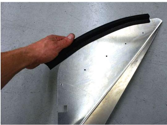
Remove the side panel then measure, mark, drill rivet locations where the  $\frac{3}{4}$ " tube is located and press on the bulb weatherstrip.
