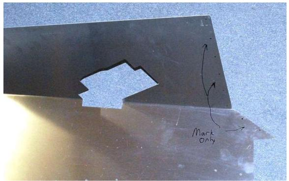
Drill the right-side floor where it was marked to attach to the chassis. Mark the two front flanges but do not drill yet.
