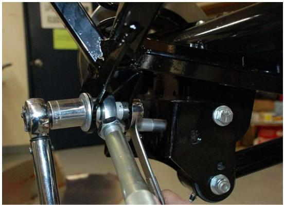
Attach the Panhard bar to the frame mount using the spacers provided.
