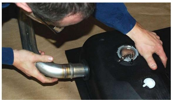
Slide the filler neck tube into the tank. A little oil or WD40 on the rubber gasket helps.
