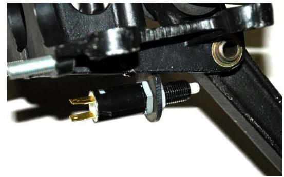
Connect the switch to the switch mount using a hex nut on each side of the mount bracket.
