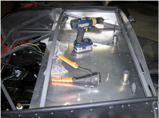
Once the panel lies flat, finish rivet it into place. The rivets along the front 2"x 3" tube should be close to the back as possible for drill and rivet gun access.
