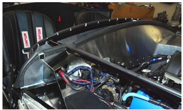
If you removed any of the other weatherstrip on the firewall or hood support tubes replace it now.
