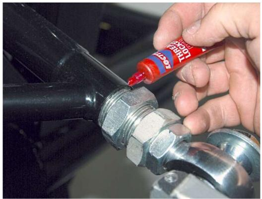
Once the car has been aligned, use a  $1^{5}/_{8}$ " wrench to loosen the upper control arm large jam nut and put some Loctite on the threads where the jam nut will sit.
