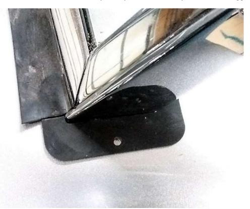
Put the rubber base plate gasket around the side bar and make sure the rubber does not go up onto the windshield bottom wipe. Trim the base plate gasket if necessary.
