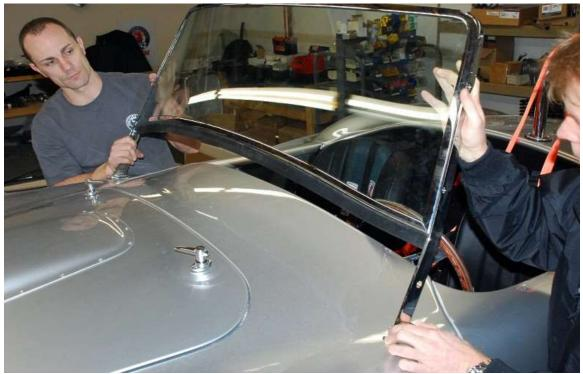
With the help of a friend, slide the windshield down through the slots in the body until the bottom seal is resting on the body.
