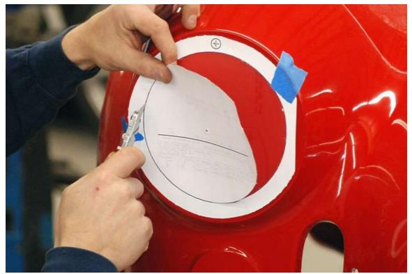
Cut the center of the template out and trace the inner circle with a marker.
