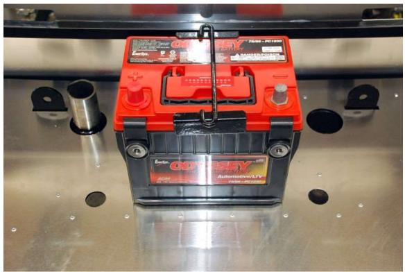
Position the battery with mounting bracket in the trunk for mounting. It is centered side to side with just enough room for the mounting bracket between it and the front of the trunk.
