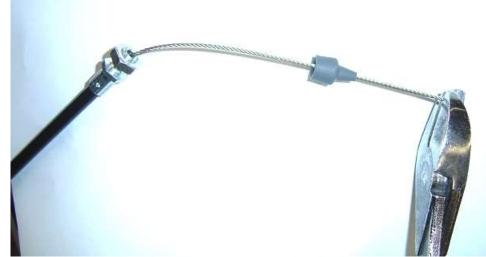
Using a pair of wire cutters, cut the barrel fitting off the cable.
