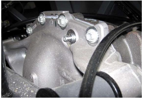
Use a hammer on the end of the barb to put the nipple in the rear cover.
