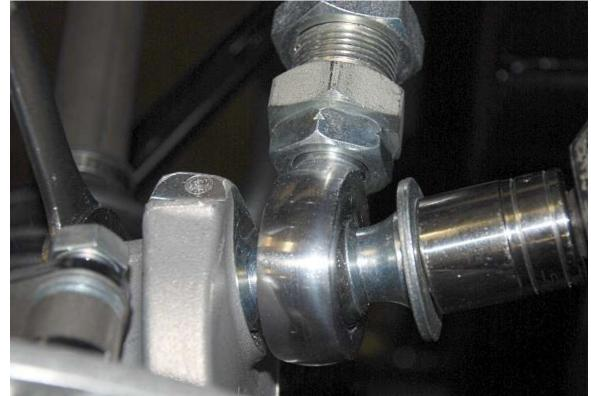
Use a  ${}^{15}/{}_{16}$ " wrench,  ${}^{15}/{}_{16}$ " socket and ratchet to tighten the locknut.
