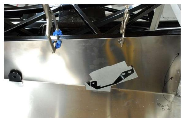
Drill and rivet the floor in place to the chassis. Use a couple clamps or tape to hold the tunnel top to the tunnel until the silicone sets.
