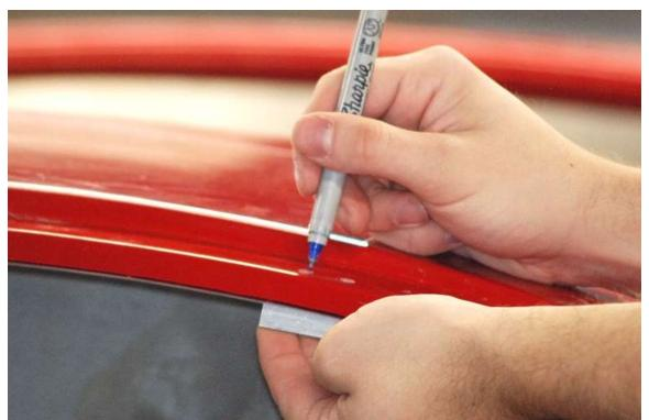
The latch brackets are in the handle assembly, center them on the line with the corner edge up against the inner radius of the hood opening and mark the two holes.
