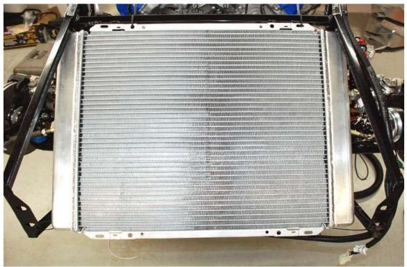
Zip tie the radiator in place on the chassis. The bottom section can just hang by a couple ties looped around the lower outlet and the drain.
