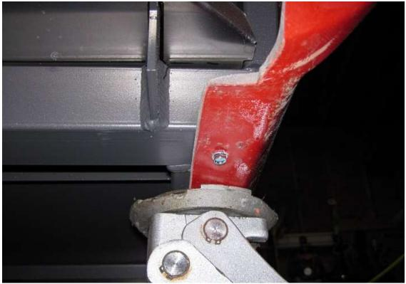
Use a jack under the side of the car to make sure the body is up against the bottom of the frame. Leave the jack so that the body can be moved in and out when pulled. Start with the body all the way in.
