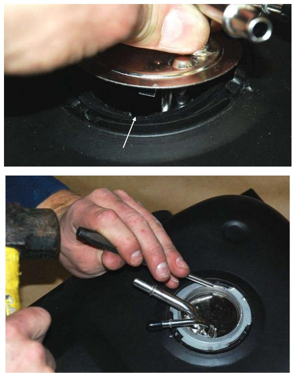
With the pickup all the way down slide the mounting collar and tap tightly into place with a punch and hammer.
