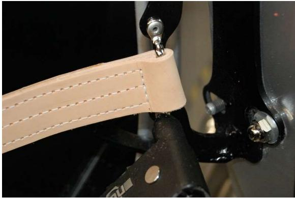
Rivet the check-strap to the door hinge using a 3/16" rivet.
