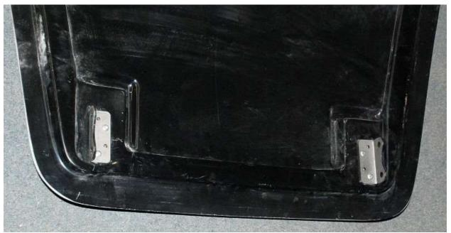
The hood hinge pivot mounts attach to the hood using rivets, the holes are predrilled in the hood liner but you may need to clean them out with a 3/16" drill bit. This is the initial install so you only need a few rivets if you are going to remove the hinge brackets prior to body painting (recommended).
