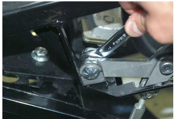
Tighten the mount bracket to fixed gear carriage bolts.
