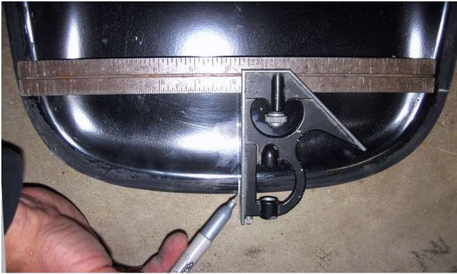
Use a square to transfer the mark to the back edge of the scoop then mark the top side of the scoop as well.
