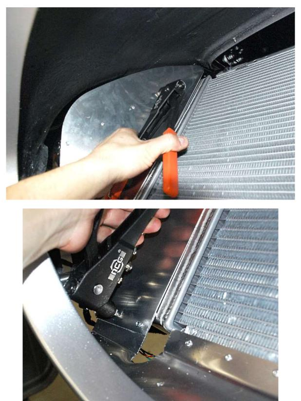
Reinsert the side panel then silicone and rivet the panel to the  $\frac{3}{4}$ " tube and the radiator floor aluminum.
