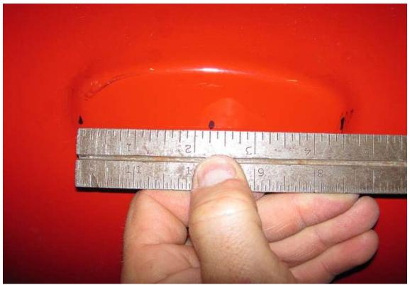
Use a ruler to measure and mark the ends and the middle of the light area.
