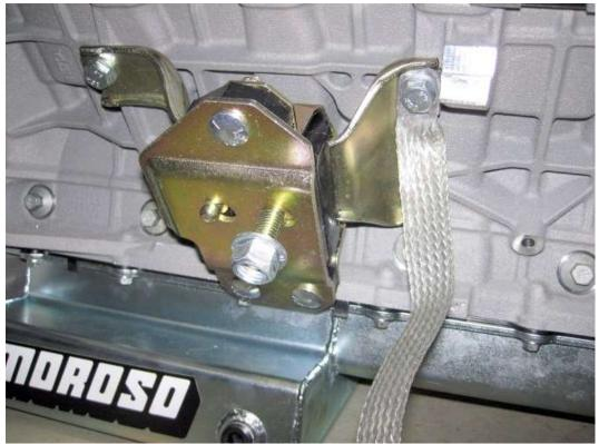
Unpack the engine mounts and attach to the engine. Don't forget to attach the engine ground strap to a right-side engine mount bolt.
