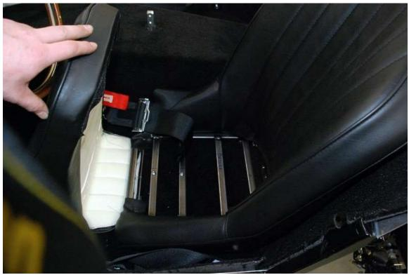
Drill back up through your seat mounting holes to put holes through the carpet and re-mount the seats.
