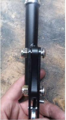
Slide the lower handle between the ratchet to handle mount plates and bolt the three pieces together using the two  $\frac{5}{16}$  x 1" button head screws as shown above. The bolt heads should be on the right so there is more clearance against the transmission tunnel.
