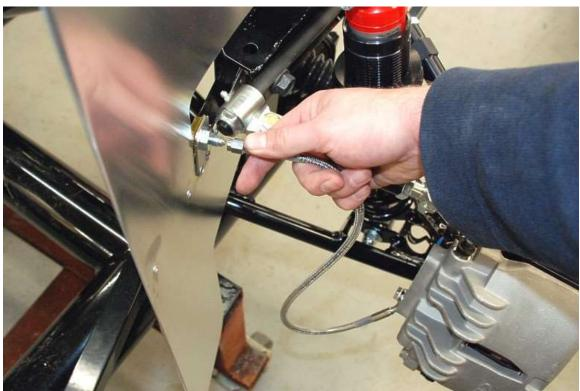
Attach the front brake line to the caliper making sure there is a crush-washer on either side of the fitting and then screw the other end of the line to the fitting on the chassis. Hand tight is fine on all these for now.
