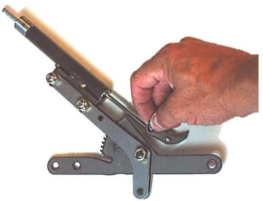
Rotate the fixed gear out of the way and pass the anchor bolt up through the lower handle.
