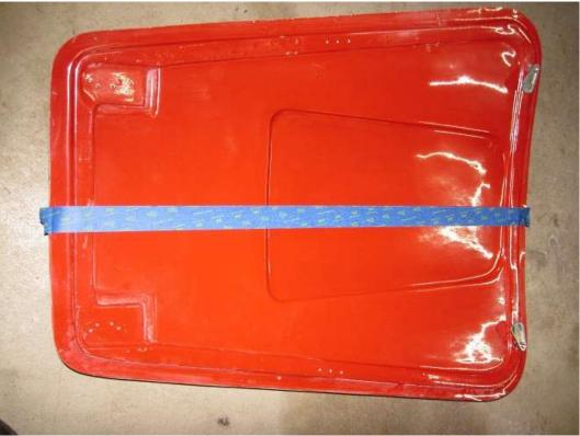
With the hood marked for its centerline, transfer this to the underside with another piece of tape.
