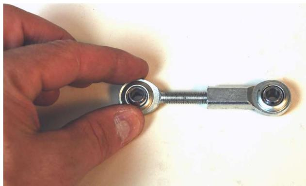
Screw the male and female rod ends together.
