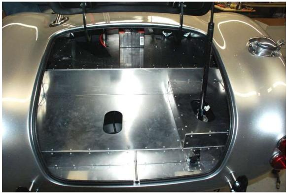
Re-mount the trunk to the hinges and re install the latch pin.
