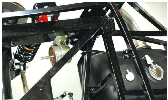
Hold the filter up to the 2"x 3" chassis tube, mark the holes, then drill and rivet the bracket on using 3/16" rivets.
