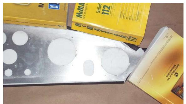
Wrap the dash pad around to the back and glue it. Use some heavy books to hold the pad in place until the adhesive has a chance to dry.
