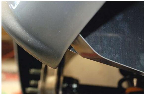
Bend the lower tab by hand to fit up flush with the body.
