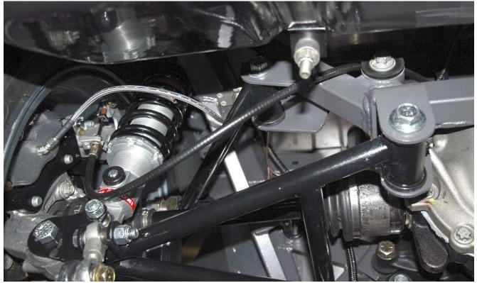
Run the left e-brake cable over the top of the center section and left rear mount then down and over to the brake caliper.
