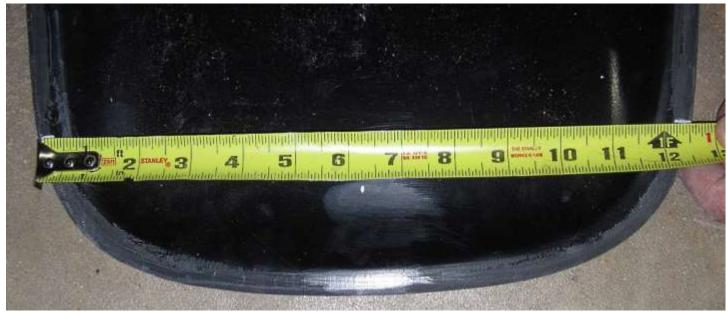
At the lines marked, measure across and mark the center of the scoop.
