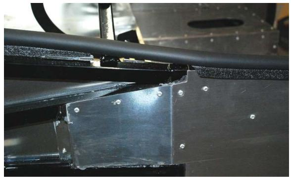
Cut out a section of the C channel where the hoop comes across to allow one piece to run the whole way.
