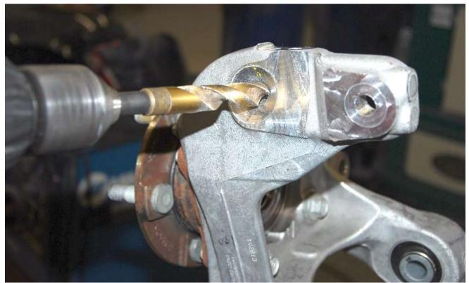
Use a  $\frac{5}{8}$  drill bit to drill out the tapered hole at the top of the spindle.
