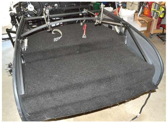
Line up the notches with the  $\frac{3}{4}$ " tubes and work forward.
