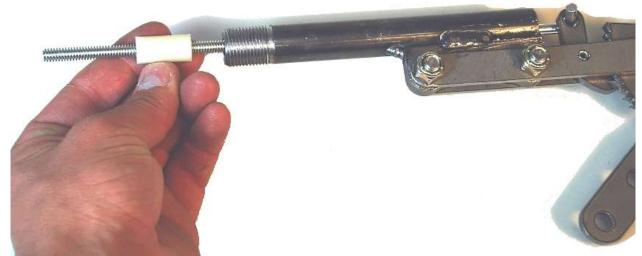
Slide the 1" nylon spacer onto the end of the anchor bolt.
