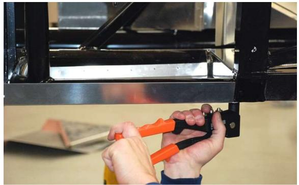
Drill silicone and install the driver's footbox floor. The outer flange does not get drilled yet.
