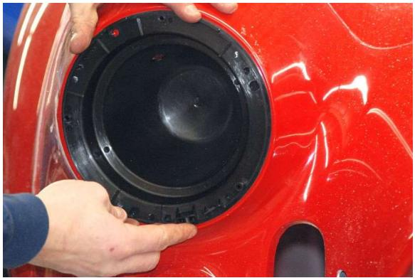
Test fit the light bucket and rubber gasket making sure that they sit flat and the bucket is centered on the fender. Mark and drill the four mounting screws for the headlight bucket using a 1/8° drill bit.
