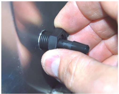
Insert the bulkhead fitting and spin the nut on the backside of the panel. Tighten the fitting using  $\frac{7}{16}$ " and  $\frac{11}{16}$ " wrenches.
