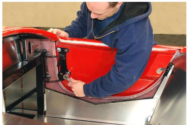
Unbolt the door from the hinge leaving the hinge attached to the chassis. Cut the zip ties in the door latch area.
