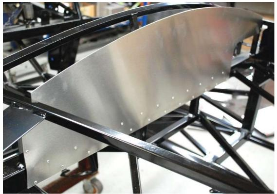
Rivet the firewall in position on the chassis.
