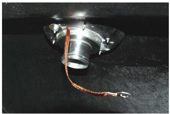
The one remaining cap fastener is a longer screw and nut used for the ground strap, screw it in from the top then put the ground strap washer and nut on from underneath.
