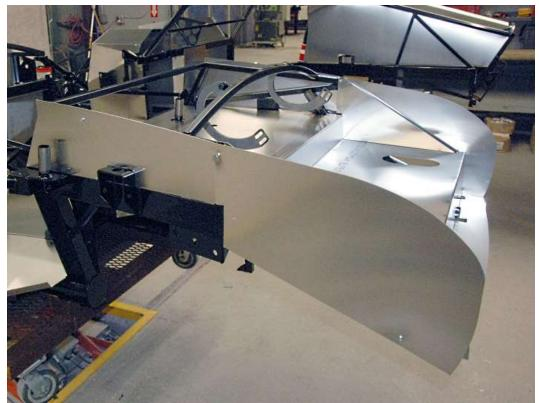
Silicone and rivet in the trunk side panels.
