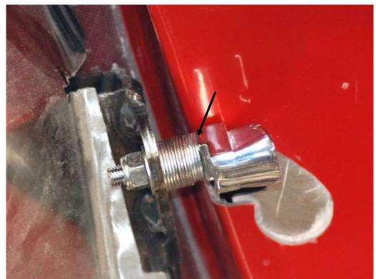
Bolt the striker onto the chassis putting enough shims on the striker to bring the base of the striker head flush with the door latch pad when the door is closed.
