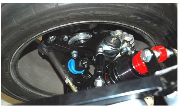
Install and torque your wheels. Make sure they rotate freely and do not interfere with the brake calipers, lines, or any suspension components.
