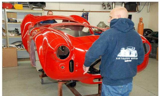
Unbolt the Quick Jacks and remove the body. Two people can do this but it is much easier with a third person to pull the sides clear of the chassis.
