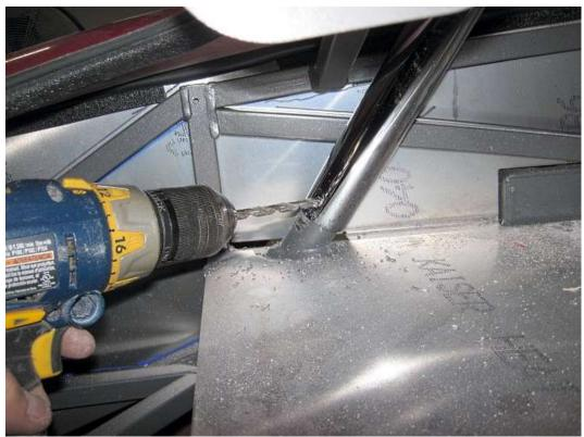
Drill the rear leg lower hole last making sure to drill through the frame mount.
