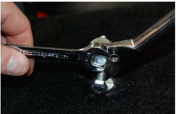
Unpack the shift handle and bolt it to the transmission. These bolts have a tendency to rattle loose so use a little thread locker.
