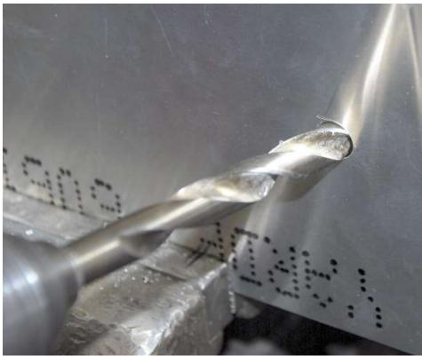
Decide the routing of your reservoir to master cylinder hose and drill a <sup>1</sup>/<sub>2</sub>" hole through the aluminum for the bulkhead fitting. The fitting is slightly larger than <sup>1</sup>/<sub>2</sub>" so wiggle the <sup>1</sup>/<sub>2</sub>" bit around to oversize it.
