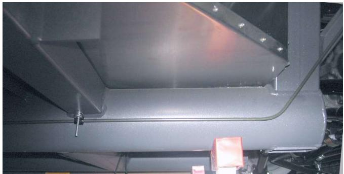
Run the brake line up the back of the 2"x 3" tube using line clips and rivets on the 2"x 2" tubes.
