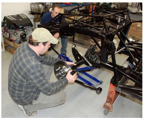
With one person holding a side of the axle raise the axle so that the lower control arms can be bolted onto the frame.
