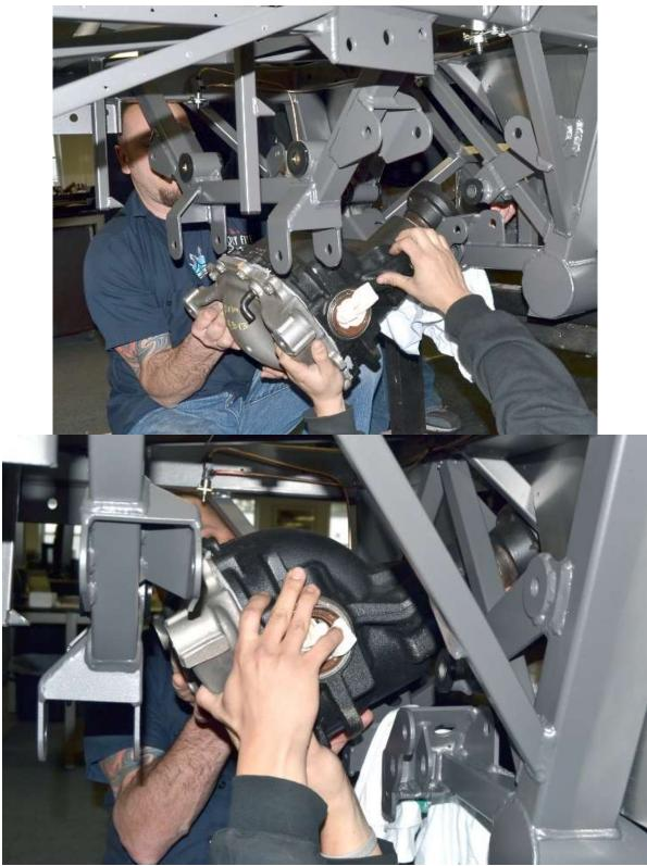
With the help of a friend, lift the center section nose up into the frame and over the front mount.
