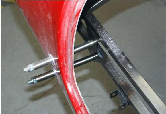
The nut and bolt use a <sup>5</sup>/<sub>8</sub>" wrench and socket to attach the rear quick jack bolts to the frame and body.
