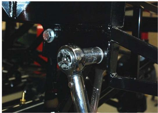
Tighten the bolts on the quad shock brackets.
