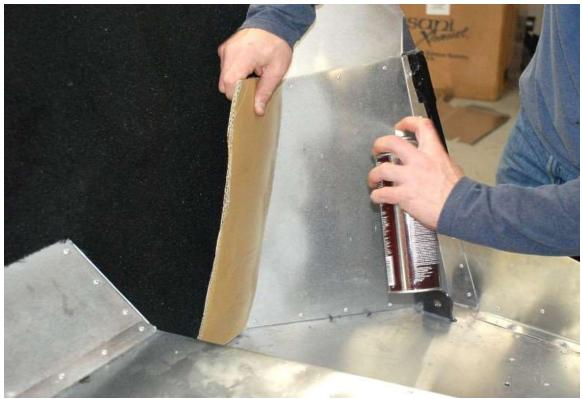
The cockpit rear corners go on next. Be very careful spraying the adhesive once some carpet is mounted. Guard the carpet with masking tape or cardboard.
