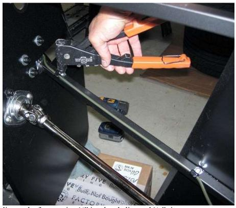
Attach the brake line to the frame using  $\frac{1}{4}$ " insulated clips and  $\frac{3}{16}$ " rivets.
