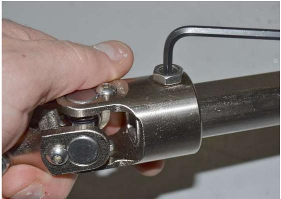
Reattach the joint to check the fit and position of the recess then remove the tube.
