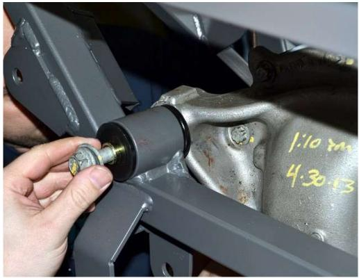
Flatten the center section out so it is horizontal then back it up so it is above the mount locations and lower it down so the bolts can be installed. The smaller/shorter bolts are used for the rear mounts.
