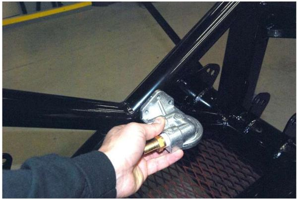
Mark the hole locations for the oil filter relocator on the old AC bracket or on the front frame X member (preferred location). If you're going to mount the relocate bracket on the X member.
