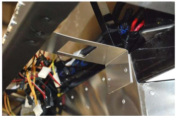
Rivet the panels to the chassis and then use the trim screws to attach them to the bottom of the dash.
