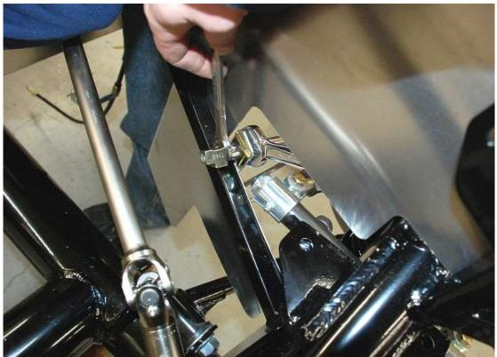
Screw the brake line T fitting into the end of the left side brake adapter and tighten with  $\frac{1}{2}$ " and  $\frac{3}{4}$ " wrenches.
