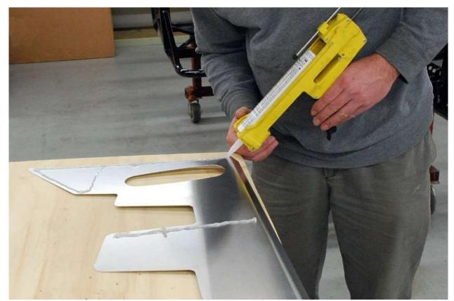
Apply silicone to the panel or chassis (whichever is easier) in the areas where they will make contact.
