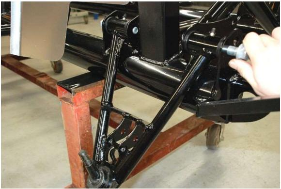
Mount the lower control arms using the outer set of holes on the chassis using the supplied hardware.
