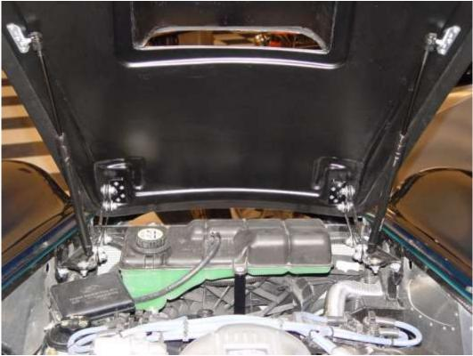
Attach the piston body end to the ball on the hood.
