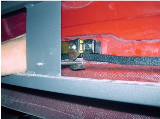
Close the trunk and test fit the latch.
