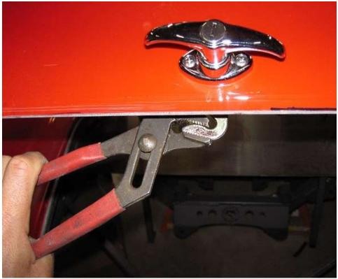
If the latch is loose, it can be bent with channel lock pliers to snug it down.
