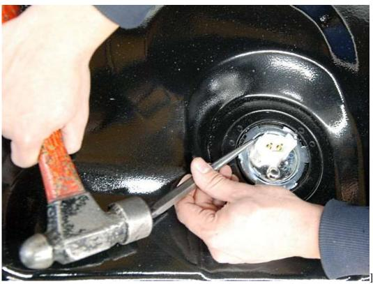
Tap the locking ring tightly into place with a punch and hammer.
