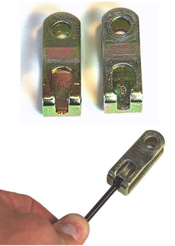
If necessary, use a drill bit and drill or a Dremel tool to open up the slot slightly.
