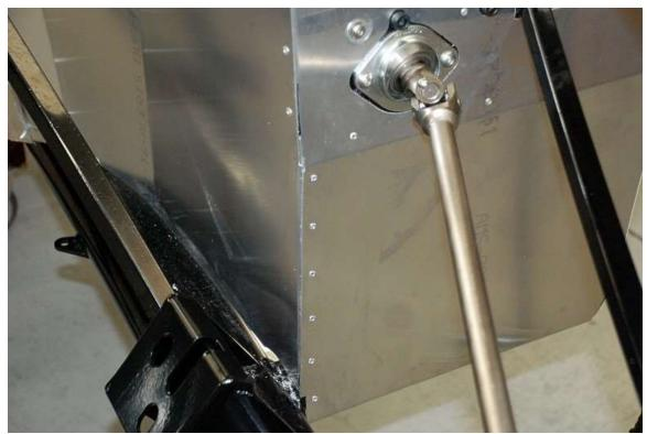
Drill, silicone and install the inner footbox wall. The front flange tucks in behind the front wall that was left unriveted. Put a little silicone on both sides of this flange.
