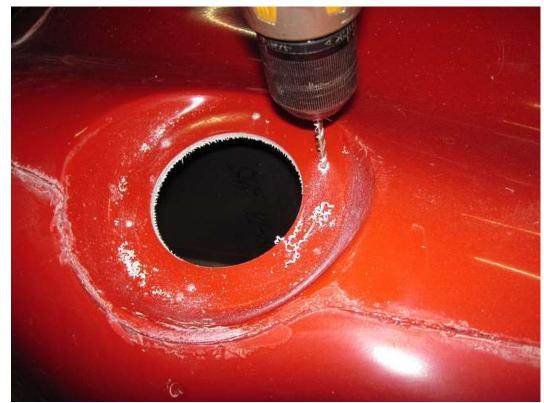
For one of the holes on the inside of the body Use a 7/32" bit drill for the grounding strap bolt.
