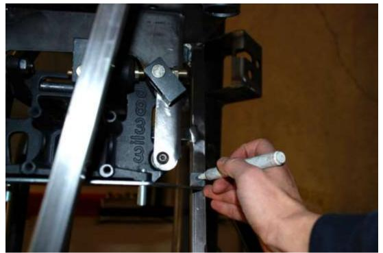
Tighten two of the front  $\frac{3}{8}$ " screws then use a marker to mark the locations of the rear mount holes on the  $\frac{3}{4}$ " tubes.
