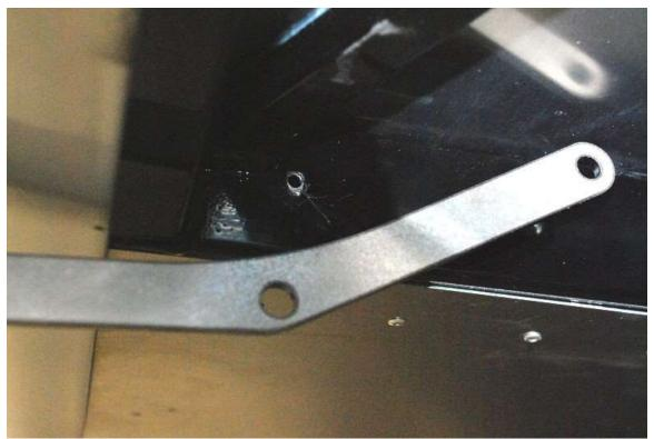
Drill a  ${}^{3}/{}_{16}$ " hole in the 2"x 2" outrigger tube directly above the middle hole in the mounting bracket. You want this hole as high as you can get it while still being able to mount the rubber exhaust hanger. About  ${}^{1}/{}_{2}$ " down from the aluminum floor.
