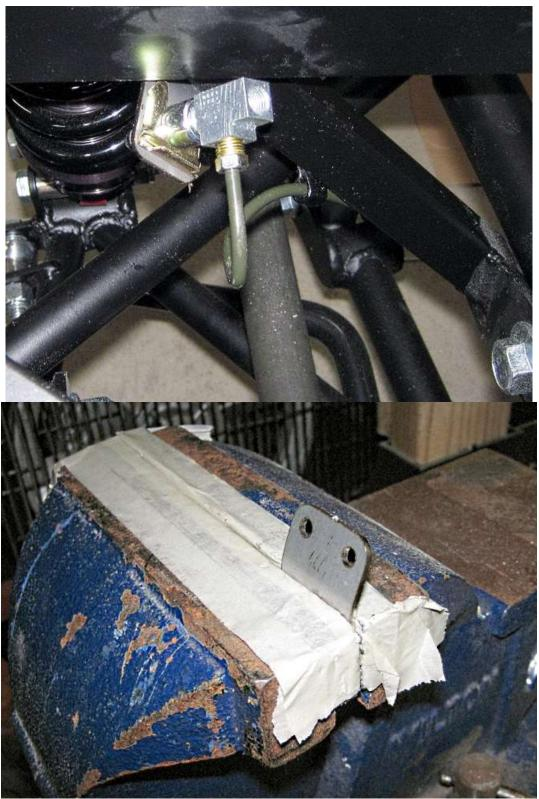
The flexible brake line mount can be on the 1" square tube but the mount may need to be bent so the T clears on the inside.
