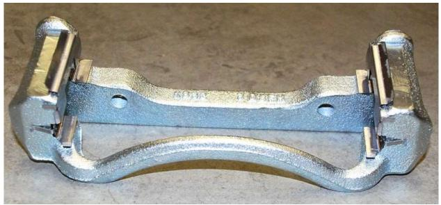
In the supplied hardware bag there are six steel clips that are designed to separate the pads from the caliper. These clips allow the pads to slide on a smooth surface and not wear on the caliper. The four clips that go on the ends of the hanger are different end to end, and must be installed with the long tab facing out.
