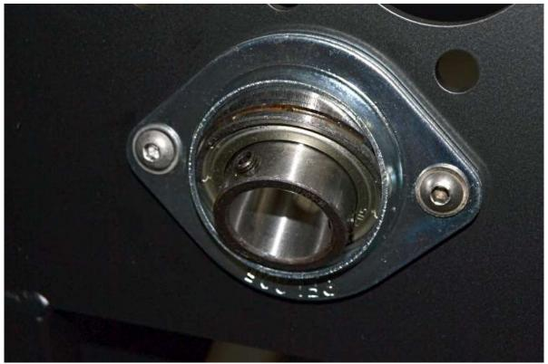
Attach the flange bearing to the front of the footbox with the set screw flange in the engine bay as shown using the  $\frac{5}{16}$ " x 1" button head screws,  $\frac{3}{16}$ " hex key and  $\frac{1}{2}$ " wrench.
