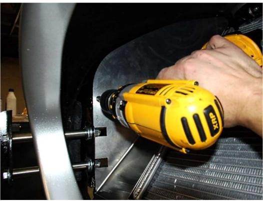
Line up the edge of the radiator fins with the edge of the side aluminum and attach the piece to the  $\frac{3}{4}$ " tube using a self-tapping screw.
