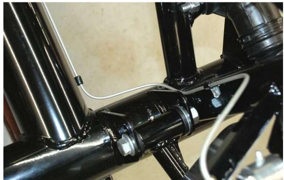
When you are happy with the routing use the small insulated line clips and 3/16 rivets to hold it in place. Mount the line clips and seal with silicone anywhere you pass into the passenger compartment.
