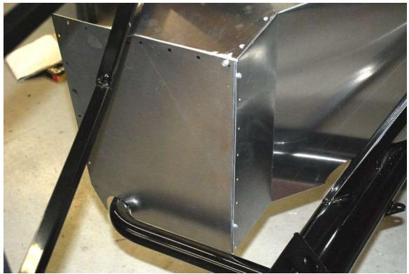
Silicone the panel and install with the temporary screws then drill through both panels and rivet it in place.
