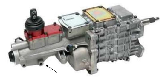
If you are using a Tremec 3550, TKO 500 or, a TKO 600 you will need to trim off the unused mounting boss on the bottom of the case.
