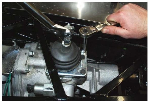
Fill the transmission with fluid and install the shifter assembly. Leave the shift handle and knob off for now.
