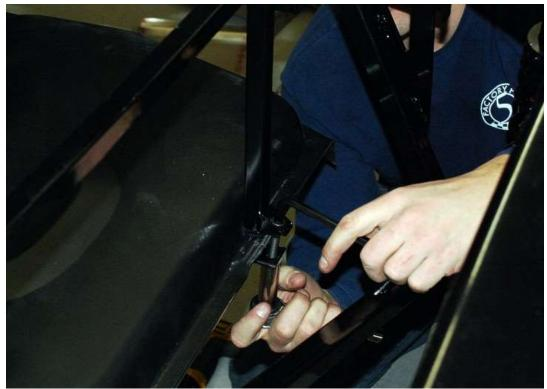
Tighten only the driver's side strap as the passenger one will be removed for aluminum fitment later on.
