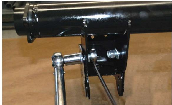
Tighten the two short bolts. Torque to Ford Specs 75-95 Nm (55-70 lb-ft).
