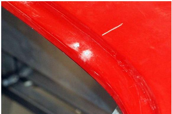
Open the hood and drill two  $_{3/16}$ " holes in the hood opening recess  $\frac{1}{4}$ " on either side of the centerline and  $\frac{1}{4}$ " back from the edge of the opening. These are for mounting the hood catch brackets.
