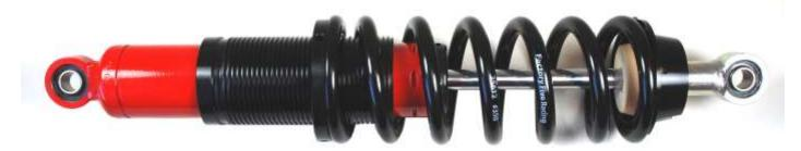
Assembled solid axle Koni coil-over shock.
