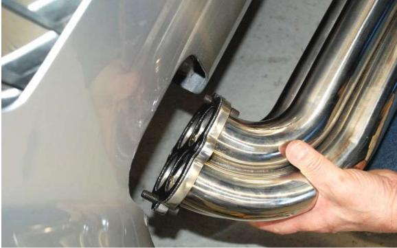
Bolt the pipe and gasket to the header or J-pipe flange with using the shorter <sup>3</sup>/<sub>8</sub>" bolts and mechanical locknuts.
