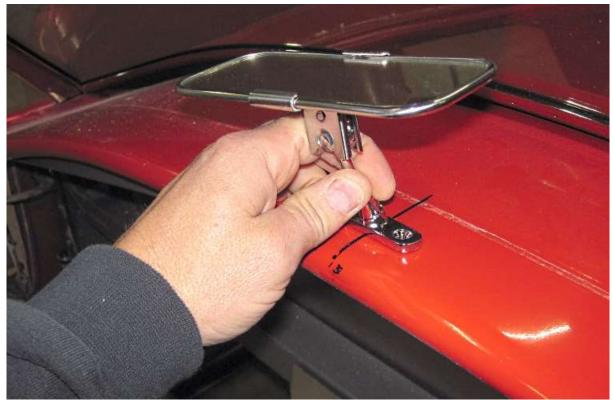
Line up the rearview mirror with the center mark and mark the holes in the body.
