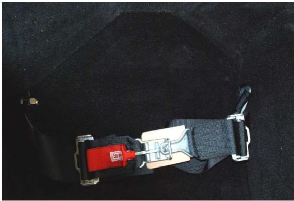
Bolt the lap harness in position with the inner most nut inside the transmission tunnel.
