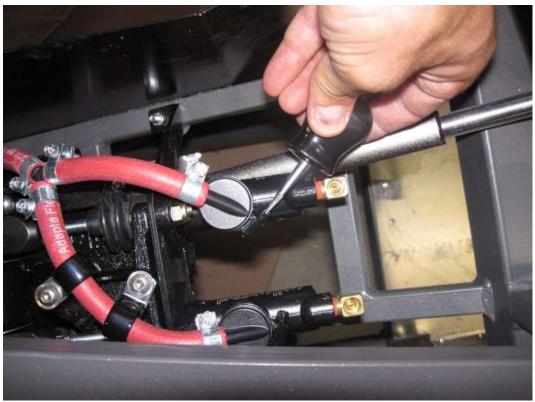
Attach the master cylinder hose adapter to the master cylinder and use insulated clips from the secondary body fasteners box or zip ties to hold the lines in place.
