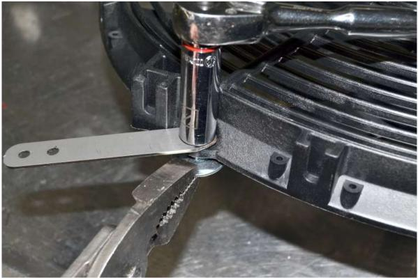
Thread on the lock nut and tighten with a  $7/_{16}$  deep socket.
