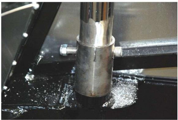
Insert one of the bolts after drilling each hole to ensure that the rollbar does not move.
