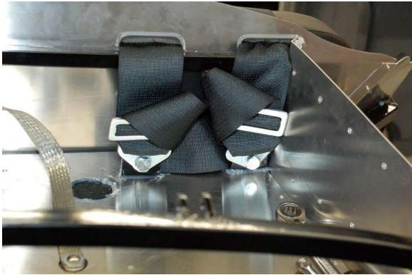
Replace the slider and mounting tab and bolt the tab to the chassis.
