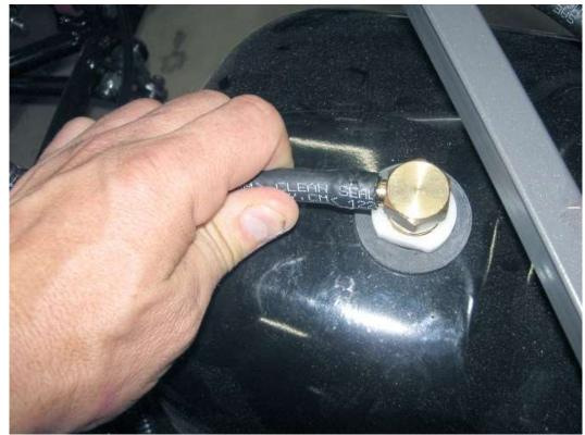
Attach a 25" section of  $\frac{5}{16}$ " fuel line and fuel line clamp onto the vent.
