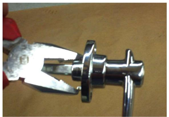
Remove the hood handles from the three-lock set and break off the bottom small tabs with a pair of pliers.
