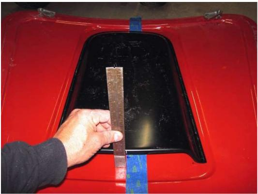
Place the hood scoop on the underside of the hood then use a square to locate the scoop left to right and the front marks to locate it to forward/backward.
