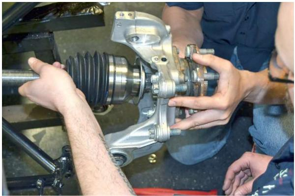
Slide the spindle onto the outer CV joint and start the nut on the end.
