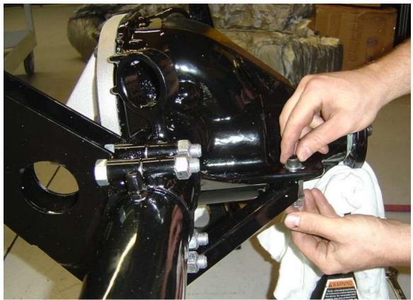
Attach the front of the upper link axle mount to the front axle flange.
