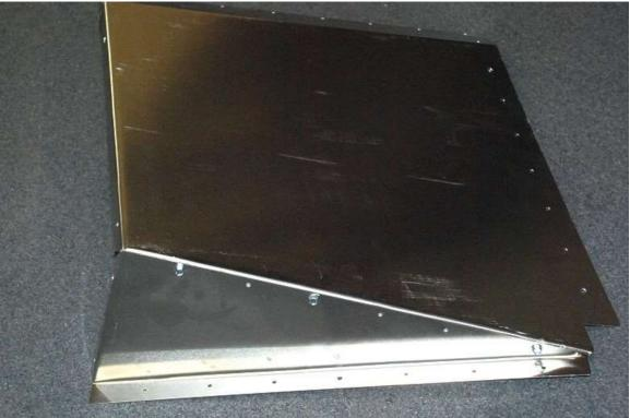
Silicone the flange between the outer top and the outer wall and attach the two pieces together using the temporary screws.
