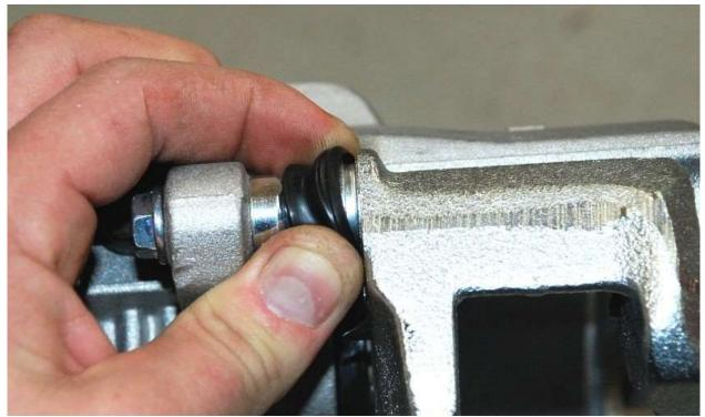
Push the rubber boots over the lip on the caliper bracket to seal the slider bolts correctly.
