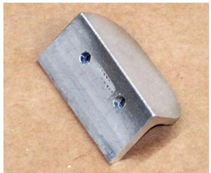
Drill the two holes just marked with a  $_{7/64}$ " bit and file the edged of the bracket round with a file or grinder for a nice finish.
