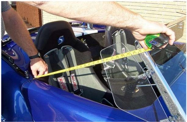
Angle the windshield so that the measurement from the center of the top side bar screw to the inside corner of the door opening is 27".
