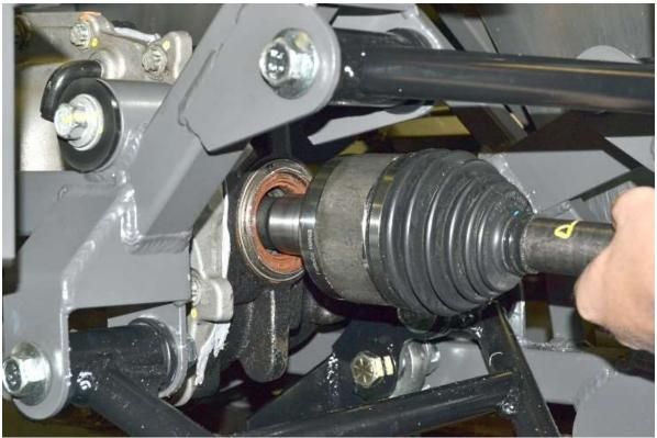
Using the correct axle, push the inner CV joint into the center section.
