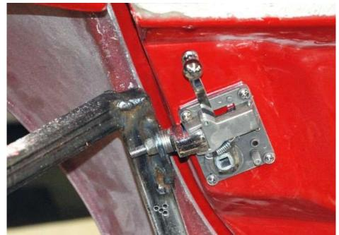
Bolt everything together to double check fit and operation. The door latches will be tight at first but break in quickly with use.
