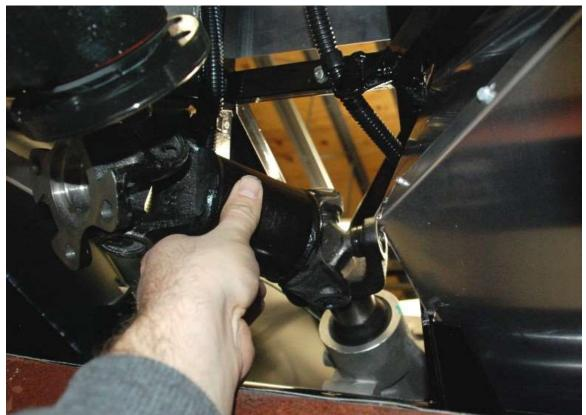
Unpack the driveshaft and slip it up into the rear of the transmission. The most room to do this is usually to hold the shaft just above the center section and come in from the driver's side.
