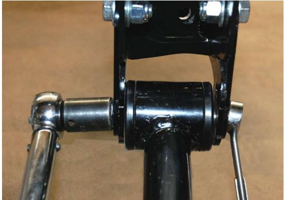
Attach the lower control arms to the brackets on the axle using the bolt provided. Torque to 101-111Nm (**75-82 lb-ft**)
