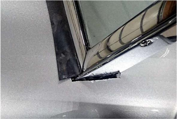
Make sure that the windshield does not hit the body on any side, if necessary, file the hole bigger.
