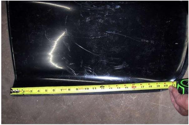
On the underside of the scoop, measure from the front back 19.50" and mark the scoop on both sides.
