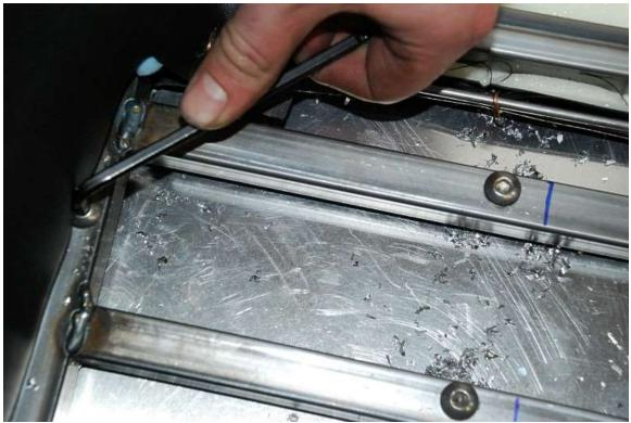
Drill the remaining holes for mounting the seats and install the bolts.
