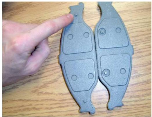
Look at the back side of each brake pad to find the inside pads and the outside pads. The difference is the location of the studs that are on the back of each pad. The studs on the inside pads are out near the ends of the pad, while the studs on the outside pads are near the middle.
