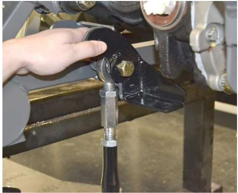
Attach the toe arms to the frame below the front lower arm mount using the  $\frac{1}{8}$ " thick spacer in the back and the  $\frac{1}{4}$ " spacer on the front side of the rod end. Use the  $\frac{5}{8}$ " x 2.25" bolts to attach them to the frame.
