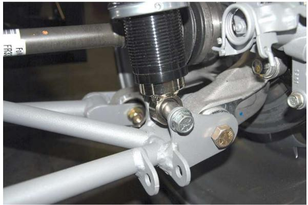
Jack the spindle up so the body end of the shocks can be mounted on the shock mount on the control arm using the longer 1.09" spacer on the back and  $7/_{16}$ " spacer in front of the shock.
