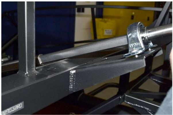
Slide the steering shaft through the upper bearing and start it in the lower shaft.
