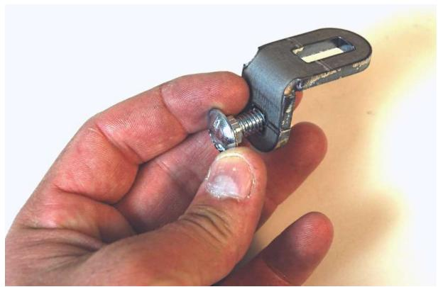
Insert a  $\frac{5}{16}$  carriage bolt into one of the bent mount brackets so the square shoulder is in the square hole.
