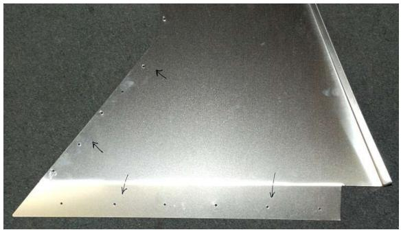
Locate the passenger footbox top and drill and mark the holes in the top flat surface only.
