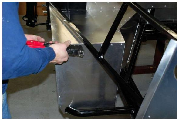
Silicone the remaining flanges then install the outer wall/top on the footbox with rivets. Make sure the rear edge is flush to the chassis and not caught up on the door hinge before you start riveting.
