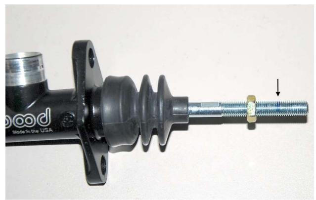
With the jam nut on the threaded shaft, cut  $\frac{5}{8}$  off each of the master cylinders.
