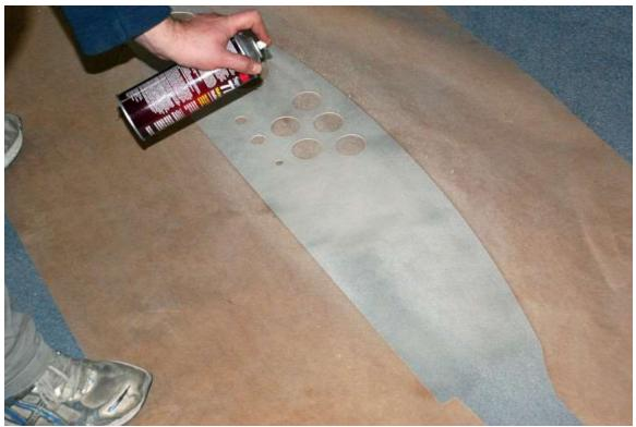
Clean the dash off with some brake cleaner or acetone and spray the front surface and the back surface of the dash pad with adhesive. (3M super 77 or super 90 work great).
