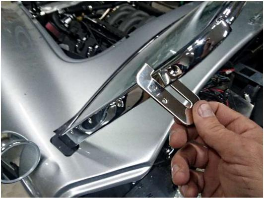
From the top, slide the base plate down to the body.
