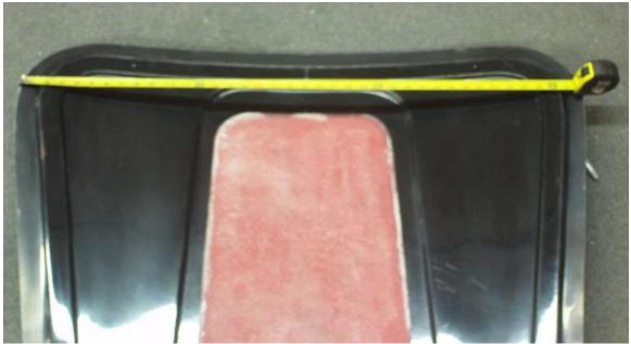
Measure the center of the hood liner rib along the trailing edge of the hood and mark it.
