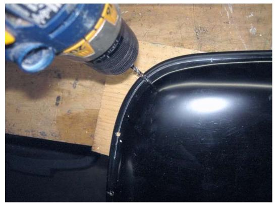
Drill 3/16" holes around the edge of the scoop.
