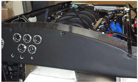
Drill for the dash mounting screws (5 evenly spread) through the dash and chassis with a  $\frac{1}{8}$ " drill bit then drill back through the dash only with a  $\frac{3}{16}$ " bit and screw the dash to the chassis.
