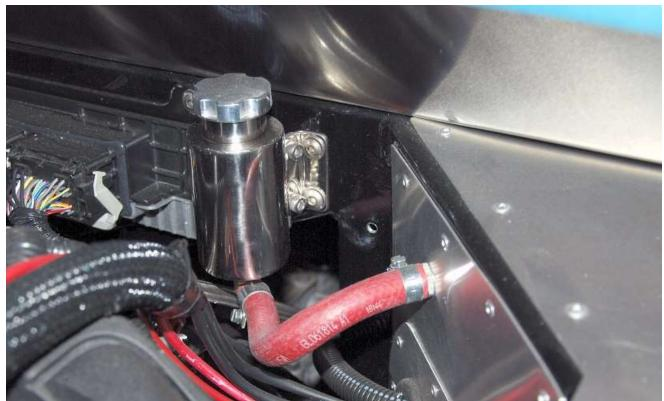
Route the hose from the reservoir to the bulkhead fitting, push a hose clamp onto the hose then onto the barb. Tighten using a 7mm socket and ratchet.
