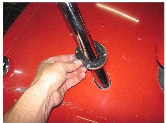
Put the rear rollbar leg through the body and onto the frame. If using rollbar grommets, put the rear ring and grommet on as well.
