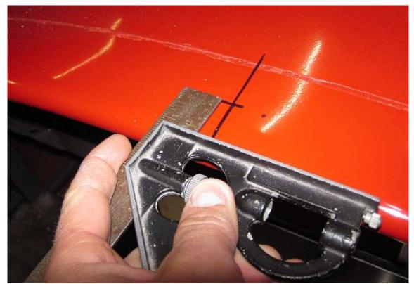
On top of the boy measure in and mark the body for the center tube location.
