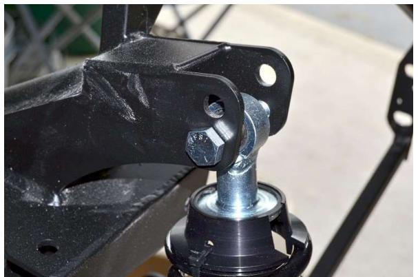
Fasten the shock to the top mount with the fasteners and 0.675" spacers provided and torque both upper and lower mounts to **40 lb-ft**.
