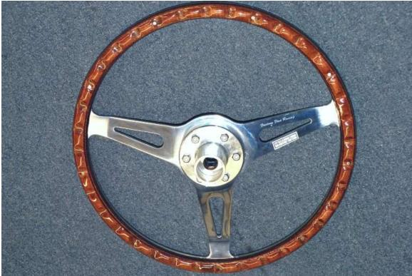
Bolt the steering wheel to the boss. The pattern is not symmetrical so it will only line up in one direction.
