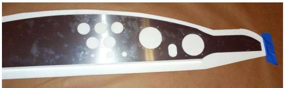
Stick the dash to the pad leaving about an inch border all around the top, the bottom will be bigger for the flange. Taping the ends of the pad helps to keep it flat.
