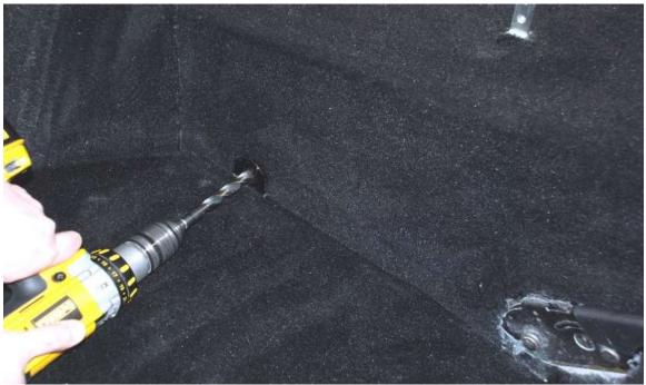
Drill through the inner lap belt mount into the tunnel with a  $\frac{1}{2}$  in. bit.
