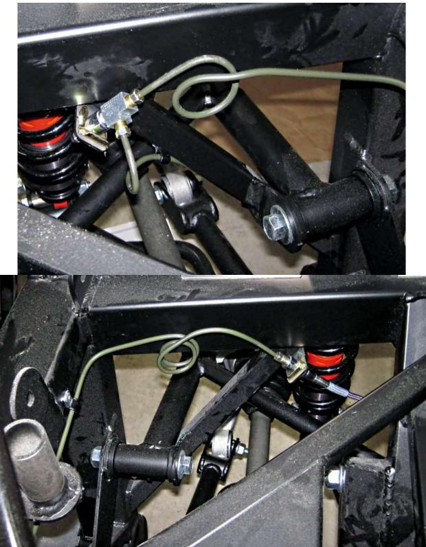
For the right side run a 60" line from the end of the left side connector then forward to the 2"x 3" tube, across and back to the 1" square tube and flexible brake line mount.
