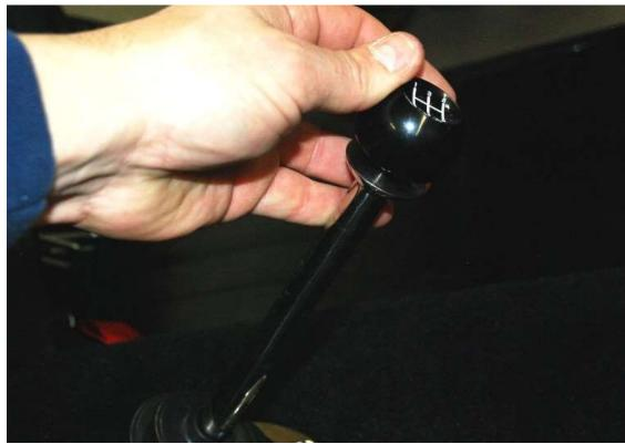
Screw the two-piece knob onto the shift handle and tighten so the shift pattern is in the correct orientation.
