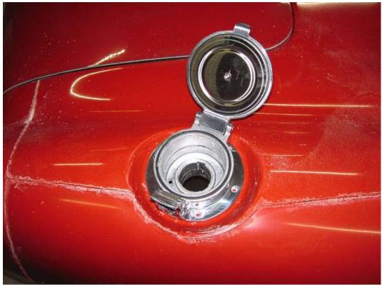
Locate the cap in the hole so that when open the cap will not hit the body and you will have access with a gas station filler handle.
