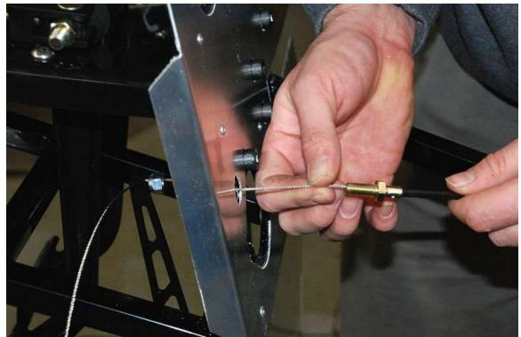
Route the cable through the hole in the firewall and slide the sheath back over the cable.
