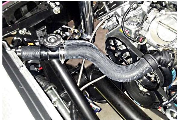
Start at the engine and route the tube above the "X" and to the upper radiator hose location.
