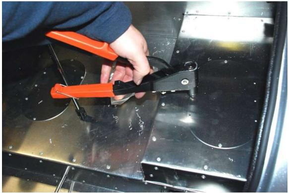
Silicone and install the patch panels in the trunk that cover the fuel sender and pickup access holes.
