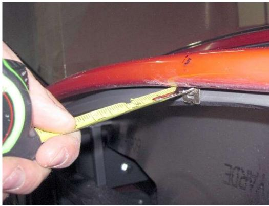
Use a tape measure to measure in from the body lip to roughly the center of the dash tube.
