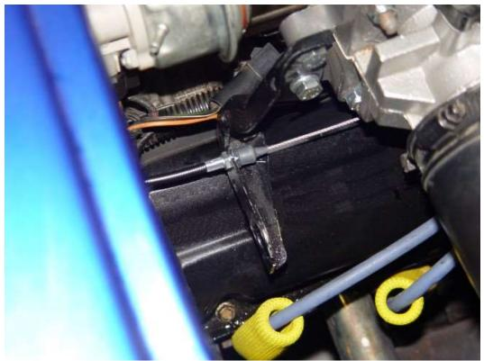
Attach the engine end of the cable sheath to the cable mount on the intake using  $\frac{3}{8}$ " and  $\frac{7}{16}$ " wrenches and push the cable wiper onto the remaining threads.
