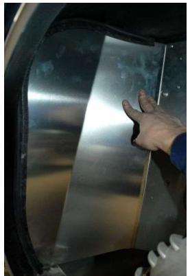
Fit the splash guards in position. If needed, trim them to fit around the outside edge, the weatherstrip will cover the trimming.
