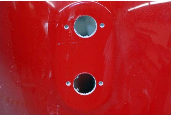
Use a 7/32" bit to drill the two outer holes for the taillight studs then cut out the center using a  $1\frac{1}{4}$ " hole saw. There are marks on the body that locate these holes. If the marks do not show there is also a template in the back of the manual.
