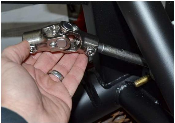
Loosen the set screw, align the set screw with the flat side on the input shaft then push the universal joint down onto the rack input shaft spline as far as possible.
