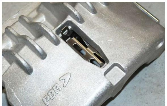
The two clips that are left go in the center of the caliper with the tab sticking up through the center hole. Insert the clip from the inside of the caliper through the large center hole with the larger tab on the side facing the pistons then press down on the outer part of the clip so the small clip goes through the large hole and clips on.
