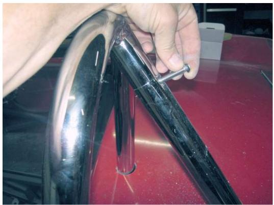
Insert the bolt through the top rollbar hole.
