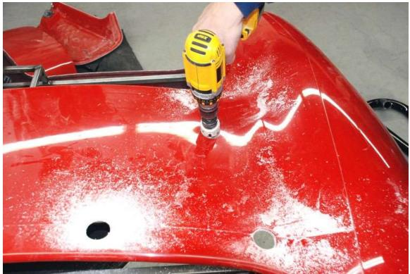
To cut the rear roll bar leg, make 2 holes overlapping so that they form the right length. Use the same  $1\frac{3}{4}$ " hole saw centered in the front of the traced opening and with the drill leaning at a  $45^{\circ}$  angle toward the inner front leg. Stop the drill when it has cut through half of the hole.
