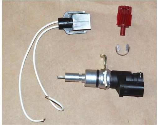
Unpack the speedometer sending unit components.
