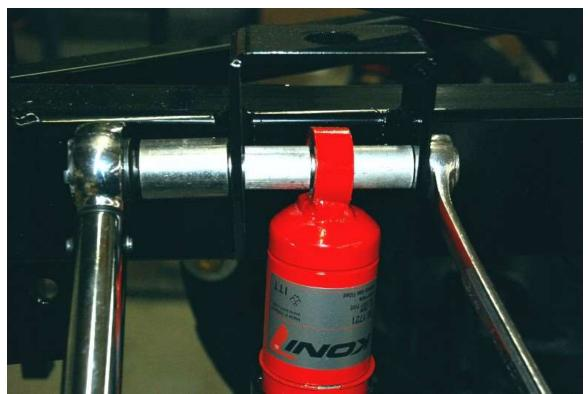
Attach the body end of the shock to the upper shock mount using the two equal length (1.09") spacers to the lower shock holes.
