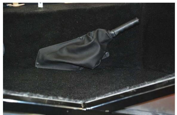
Fit the boot over the handle and check the handle actuation. When you are in a position where the boot clears the handle movement drill through the material into the tunnel and screw it into place.
