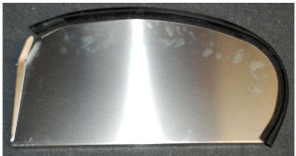
Push a piece of the bulb seal weather stripping around both rear splash guards where they will contact the body.
