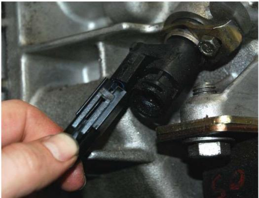
Connect the plug and plug it into the sender. If you are running fuel injection you may also need to send this signal to the computer as well depending on your system.
