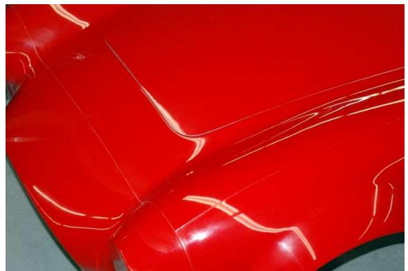
The hood has been trimmed slightly oversized to allow the panel gaps to be sanded down to fit. Set the hood in place and make sure it will fit the opening in the body, if needed sand or file the edges to allow the panel to just fit with a very small gap all around.
