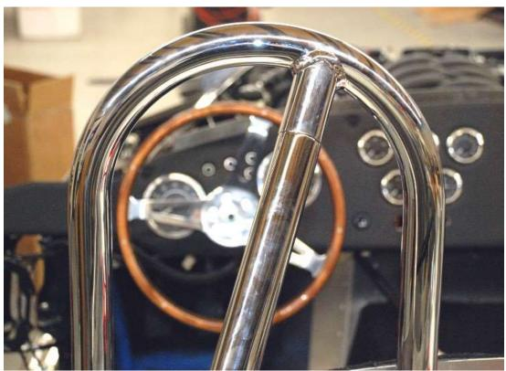
Slide the rear leg up over the mount on the hoop and make sure it comes all the way up flush. Clamp the rear leg up with a pair of vise grips. The front hoop will angle back about  $6^{\circ}$  or so.
