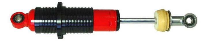
Slide the coil sleeve over the body of the damper beginning at the end which has the rubber bump stop. The unthreaded end of the sleeve goes first so that it will sit on the snap ring on the shock body.
