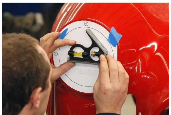
Cut out the headlight templates from the back of the manual on the outermost diameter and tape them in the center of the fender with the line level with the ground.
