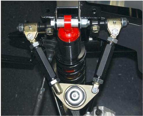
Mount the upper control arms to the chassis with the grease fittings pointed up. Use the mount holes that are vertical on the side of the 2"x 3" tube, not the top horizontal ones.
