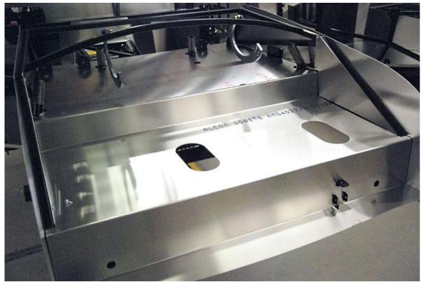
With the rear taillight harness tied up and secure, silicone and install the lower trunk floor.
