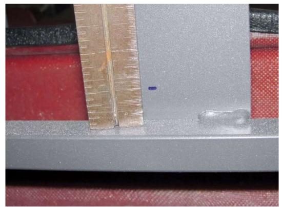
Transfer this measurement to the backside of the plate. Do the same for the side location.
