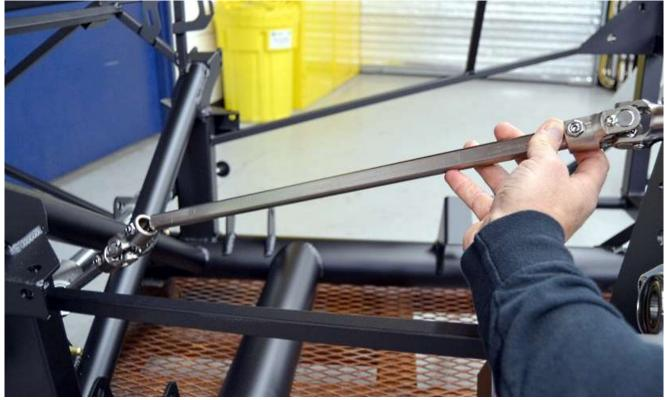
Insert the lower shaft into the steering rack joint.
