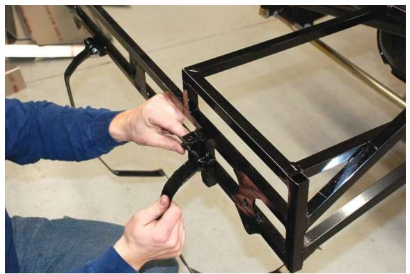
Hang the fuel tank straps from the rear mount of the chassis using two of the strap fasteners. The longer strap goes on the passenger side.
