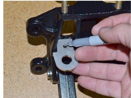
$\mathbb{V}$  The clutch switch mount attaches the same way as the Brake switch mount.
