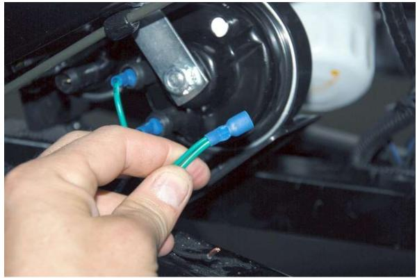
Twist the chassis harness green wire and small wire ground together and insert them into one of the  $\frac{1}{4}$ " female connectors included with the horns then crimp the connector on.
