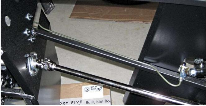
Run a 60" brake line from the front master cylinder out the front of the pedalbox along the  $\frac{3}{4}$ " tube to the front left brake line mount.
