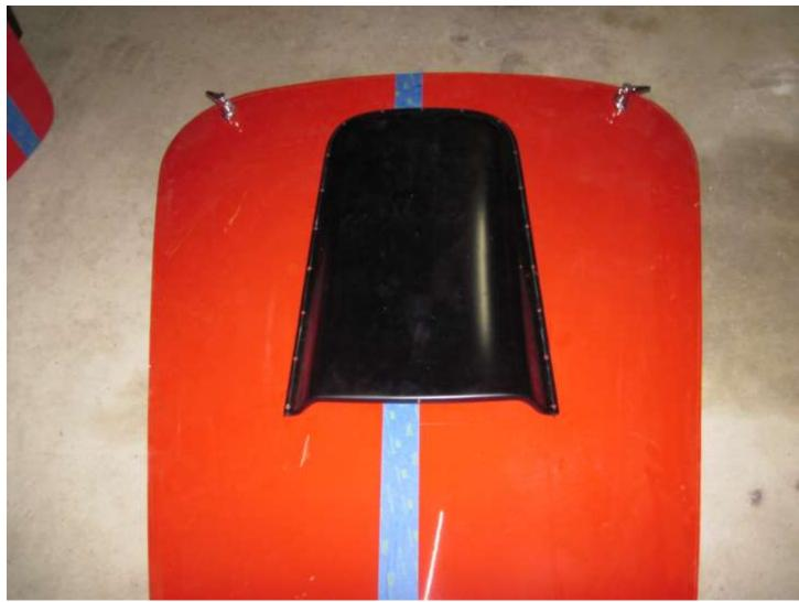
Locate the scoop using the straight edge and two marks.
