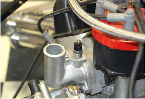
In your engine block or cylinder head, locate a coolant access point to install the thermostat switch and screw it in.
