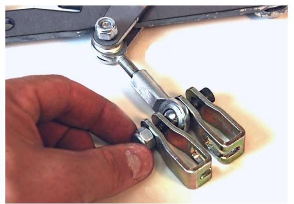
Facing the cable slots towards each other, attach one of the cable clevises to each side of the female rod end using the  $\frac{1}{4}$ "x 1.50" socket head bolt and locknut. Just start the nut for now, do not tighten it.
