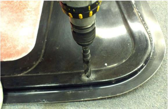
Drill through the hood and the liner starting with smaller bits working up to a <sup>5</sup>/<sub>8</sub>" hole. The larger bits sometimes work better by running the drill in reverse so they do not tear the fiberglass.
