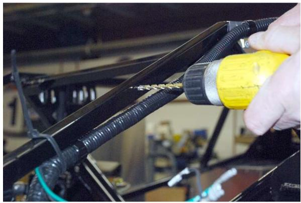
Locate the horns on the upper radiator down tube and drill a  $3/_{16}$ " mounting hole.
