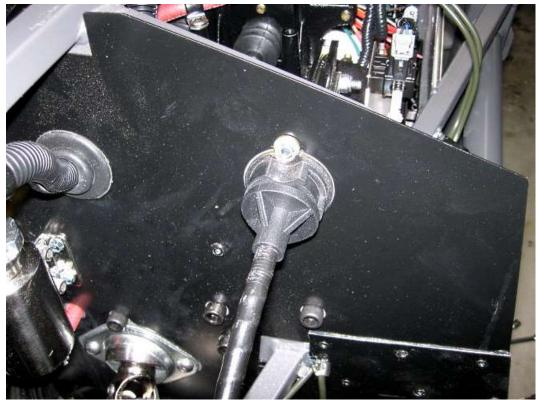
Attach the clutch cable to the firewall spacer using the small #6 screw provided and 1/4" wrench.
