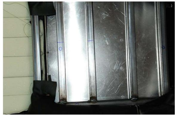
Using the rivet heads as a guide mark where the rails of the seat frame are above the seat mounting plates.
