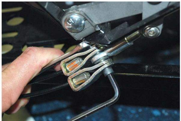
Reinstall the clevises and <sup>1</sup>/<sub>4</sub>" bolt then tighten the bolt so that the clevis ends are closed, this will prevent the cable ends from coming out.
