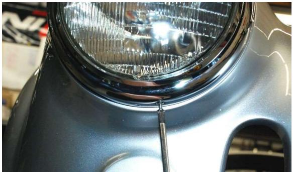
Mount the trim ring hooking it over the bucket on the top and screwing it into the bottom using the countersunk screw.
