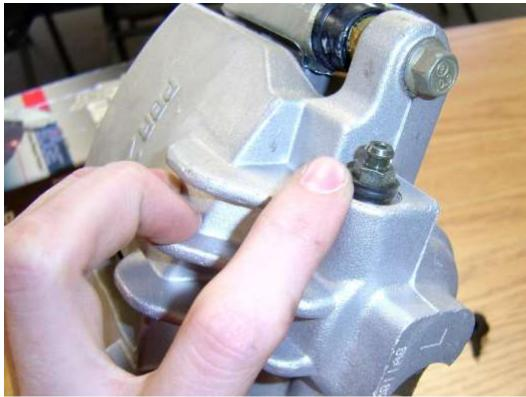
Install the caliper on the spindle; make sure that the fluid bleeder is at the top of the caliper. Torque the caliper mounting bolts to **130Nm (95 lb-ft**).
