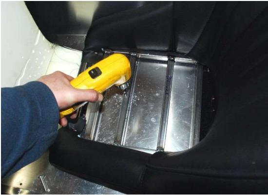
Drill the first hole for the seat mounting and install the bolt.
