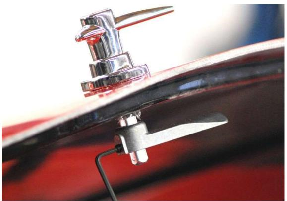
Attach the cam wedge to the underside of the hood handles and adjust for tightness using a 2.5mm hex key.
