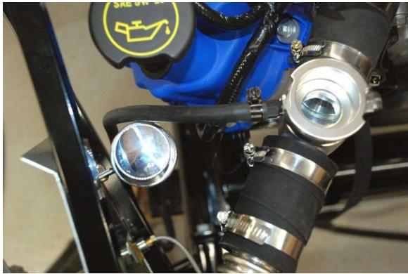
Route the overflow hose from the filler to the overflow tank.
