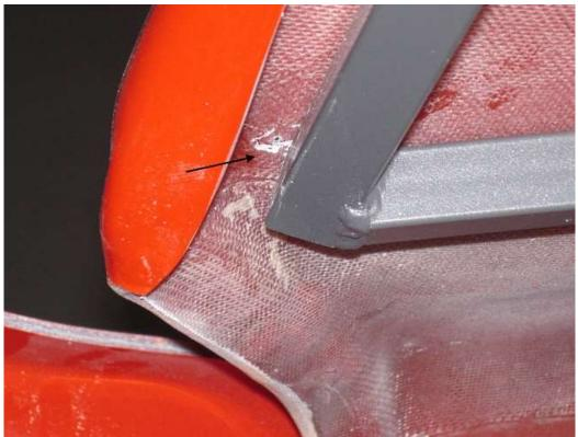
Check the outside corners of the dash tube. Make sure there is a  $\frac{1}{2}$ " or so gap between the body and frame. Try pushing down on the body here, it should move.
