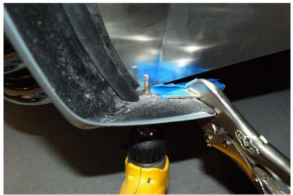
Use one of the  $\frac{3}{16}$  rivets to attach to the bottom of the fender just forward of the exhaust cut-out.
