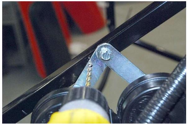
Attach the two horns to the radiator down tubes using a supplied #14 screw. Then drill a second  $\frac{3}{16}$ " hole so the horns will not rotate.
