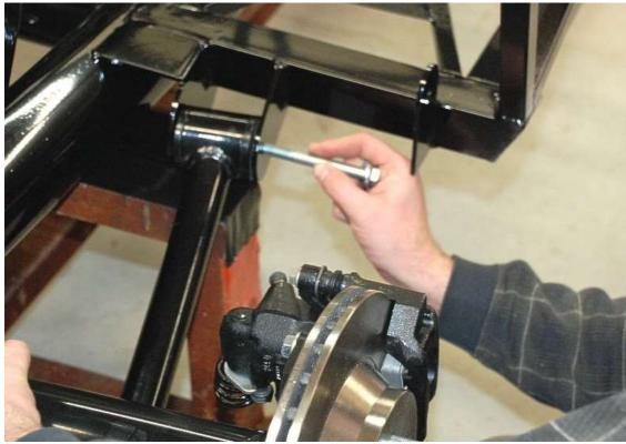
Attach the lower control arms to the frame mounts.
