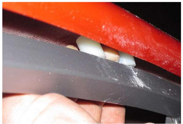
Put the plastic spacers between the dash tube and the body so the screws can go through them. 473
