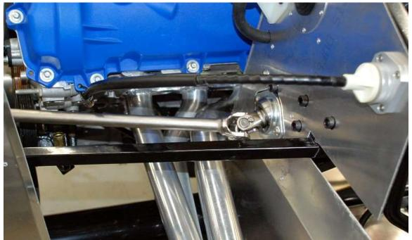
Route the clutch cable down to the bellhousing. Using zip ties or insulated clips tie the cable safely away from the headers and the moving steering components. It can be fastened to the engine using the bracket on the cable to the front lower bolt that holds the starter cable just before it leaves the block or, to the lower engine bay  $\frac{3}{4}$ " tubing.
