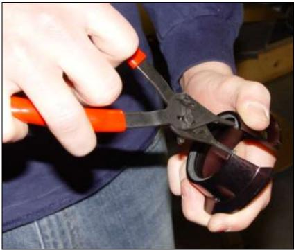
The coil-over hats have a snap ring which holds it in place. Remove this snap ring to assemble the coil over shock.
