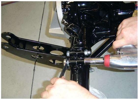
Test fit the two halves of the upper arm mount together. If it is hard to put all of the bolts in the mount holes, put in as many as you can then use a  $\frac{1}{2}$  drill bit through the remaining bolt holes.
