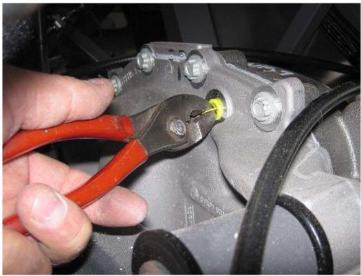
Remove the plug at the top of the rear cover.
