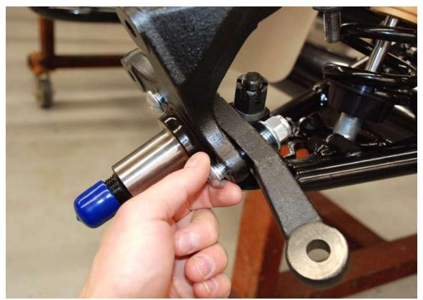
Bolt the steering arms to the spindles so the tie rod end will mount from the bottom. Torque to **60 lb-ft**.
