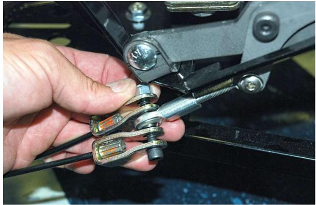
Put the locknut back on the <sup>1</sup>/<sub>4</sub>" bolt hand tight.
