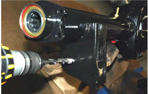
Drill the lower control arm mount holes with a <sup>1</sup>/<sub>2</sub>" drill bit.
