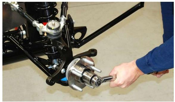
The hub is a snug fit on the spindle and may require a light tap with a soft mallet to get in place. Torque the hub nut to **305-338Nm** (**225-250 lb-ft**).
