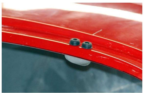
The four remaining screws are used to hold these brackets in place. They can either be countersunk into the body or used to hold down the hood bumpers to hide them completely.
