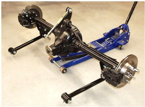
Use a floor jack to position the rear axle assembly under the frame.
