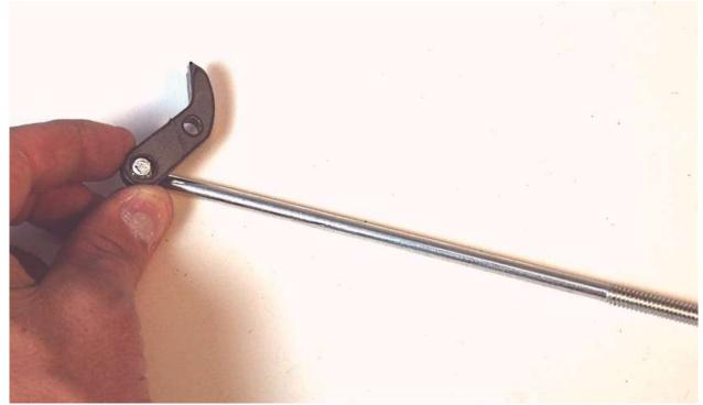
Put the ratchet tooth on the long anchor bolt as shown in the picture below.
