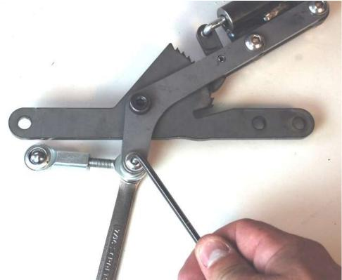
Slide the male rod end between the ratchet to handle mount plates and attach it using the <sup>1</sup>/<sub>4</sub>" flange head bolt and locknut.
