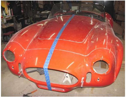
Use the outside radius of the headlight area to measure across and find the center of the body on the front deck.
