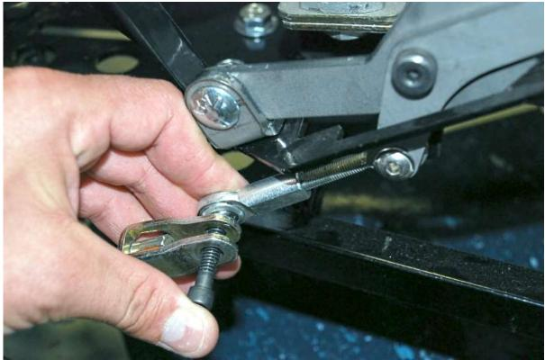
Adjust the rod end so that the <sup>1</sup>/<sub>4</sub>" bolt goes through the rod end and both clevises and the cable is tight.
