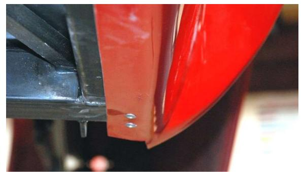
Once the body is painted and final mounted rivet the bottom lip of the body to the chassis using the long  $3/_{16}$ " rivets.
