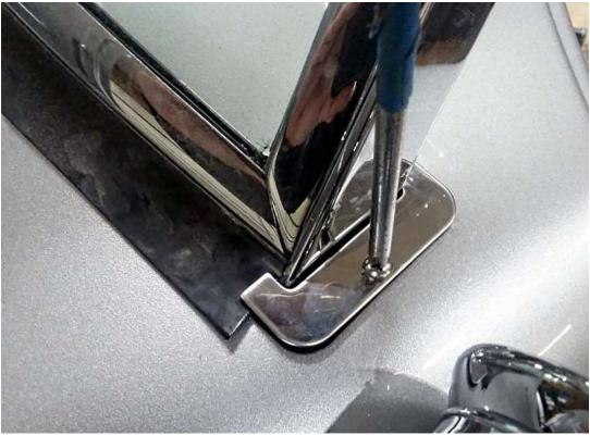
Remount and screw the base plate to the body.
