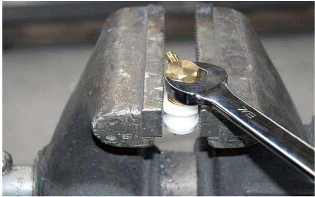
Screw the vent into the plastic bushing and tighten with a 7/8" wrench.
