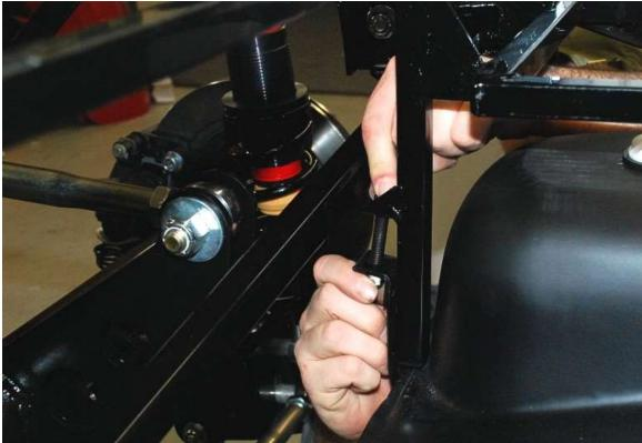
Bolt the straps in with the strap fasteners and drop the jack.
