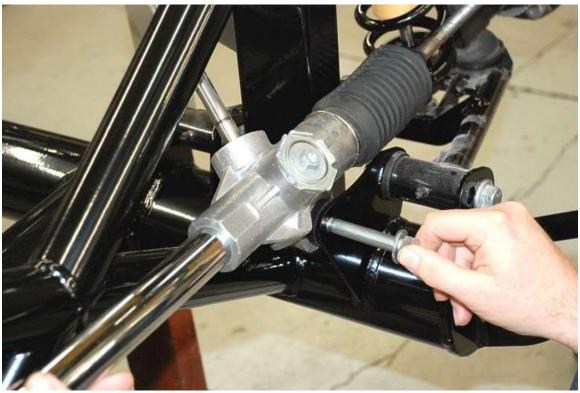
Bolt the rack into the frame. It is easier to do the driver side first then swing the passenger side down into the mount.
