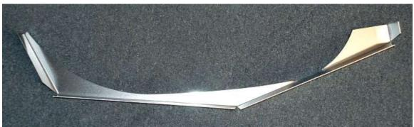
Unpack the under-door aluminum panels. They are shaped to fit around the bottom of the door with flanges to mount to the chassis.
