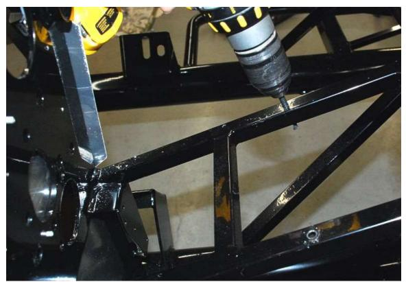
Loosen the bolts and remove the pedal box assembly from the footbox then use a  $\frac{1}{4}$ " drill bit and drill to drill through the  $\frac{3}{4}$ " tubes at the locations marked for the rear mount.
