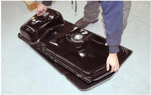
Put the metal tank in the plastic tank cover.
