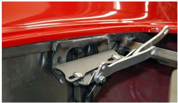
Leave the bolts loose enough so that the hinge assembly can be positioned to match the hood.
