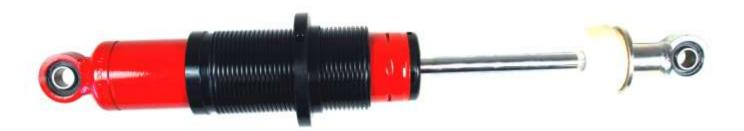
Slide the coil sleeve over the body of the damper beginning at the end which has the rubber bump stop. The unthreaded end of the sleeve goes first so that it will sit on the snap ring on the shock body.
