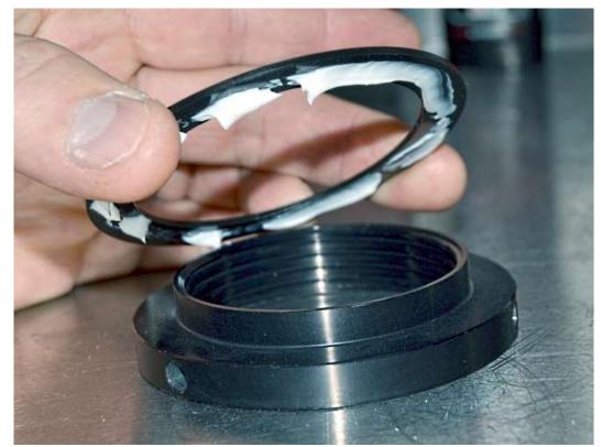
Put the Delrin spacer grease side down onto the spring seat on the threaded tube (shown without tube)
