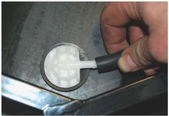
Attach the two-foot section of <sup>1</sup>/<sub>4</sub>" rubber fuel line to the fuel tank vent and run the line up high under the upper trunk and tie in place.
