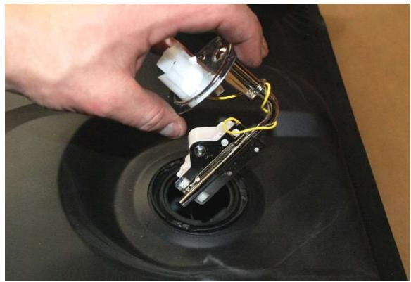
Insert the fuel level sender into the tank.
