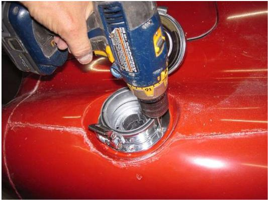
Use an <sup>1</sup>/<sub>8</sub>" drill bit through the flange holes to mark all of the outer screw holes on the body.
