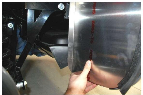
Fit the panels in place and trim the outside perimeter if needed. The small tab on the bottom faces towards the rear of the car and is on the bottom. The bent edge should be vertical and aligned with the trunk side pieces where they drop down, behind the quad shock mounts. It should sit on top of the  $\frac{3}{4}$ " vertical tube that is behind the trunk wall. You may also need to bend the flange of the gas tank down a little to get the panel in place.
