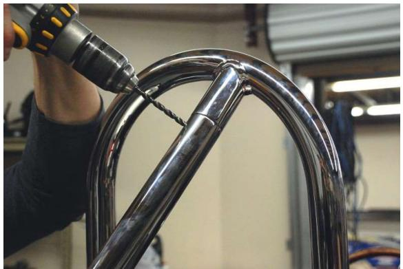
Make sure the rear leg is tight up against the main hoop and drill the upper hole. This bolt will be visible so keep this in mind when deciding the orientation. Install the bolt loosely to keep the leg in place.
