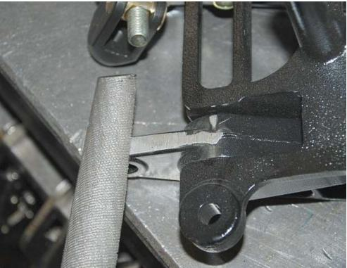
If necessary, use a file to remove the forging centerline so the 3/8" bolt can go through the clutch pedal hole.
