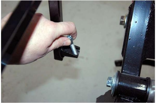
Put the Fuel tank bolts in the gas tank front frame mounts.
