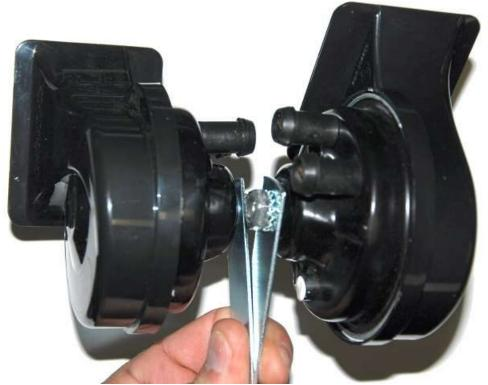
Holding the horns, the connectors should be spaced so that the wires will not hit each other.
