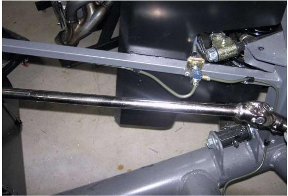
Attach the brake line to the end of the T.
