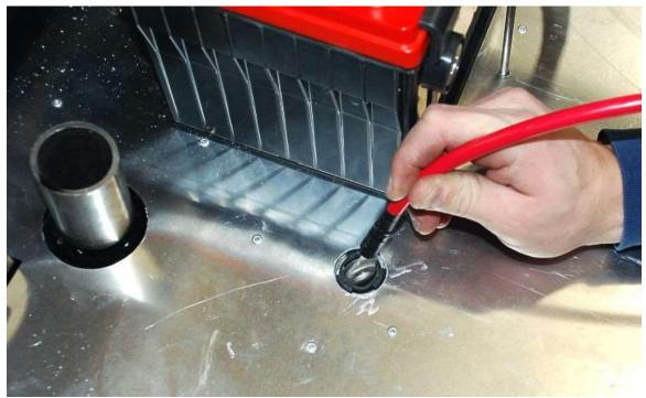
Push the small end of the battery cable through the floor from the top.
