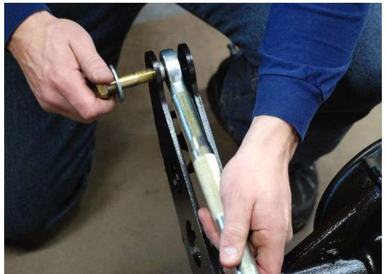
Attach the short upper link tube to the axle upper link mount using the <sup>1</sup>/<sub>4</sub>" spacers on either side of the rod end.
