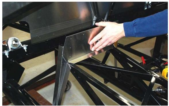
Drill the tunnel front A-shaped piece where it meets the chassis and silicone and rivet it in place.
