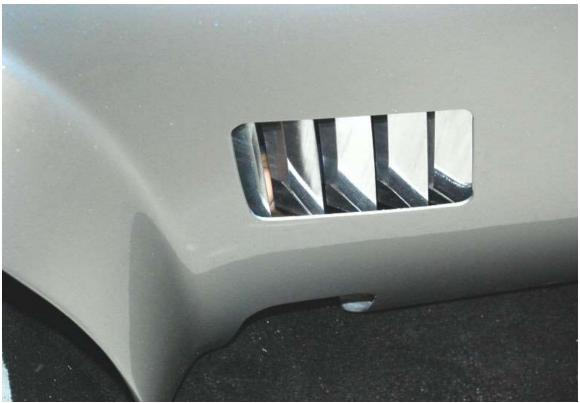
Hold them up to the body to see how they fit. They are designed to allow air to exit the engine bay so the flanges point from the rear edge in.
