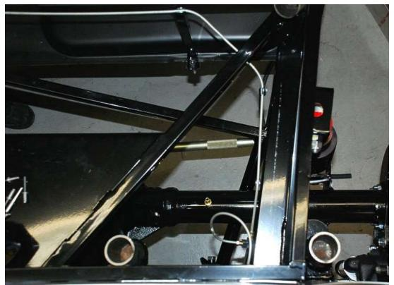
Run a 60" brake line from the "T" up the  $\frac{3}{4}$ " tube to the front fuel tank mount tubes and over to the passenger side  $\frac{3}{4}$ " tube. An alternative to running it this way would be to run it across the backside of the 2"x 3" tube.
