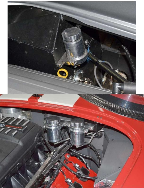
Find a location for the brake reservoir, it can mount to the front of the footbox just inside the hood opening or behind the engine on the firewall but this would require making a bracket. Use the reservoir with cap and locate it so the reservoir cap can be removed and filled with the body on.
