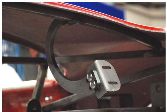
Hang the hinge arms on the chassis using the shoulder bolts. You do not need the nuts for just doing fitment.
