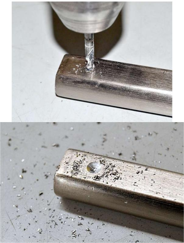
Use a  $\frac{3}{16}$ " drill bit followed by a  $\frac{5}{16}$ " drill bit at the point marked to create a slight recess for the set screw.
