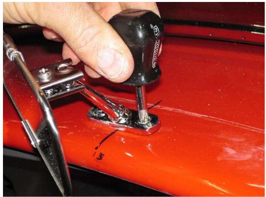
Put the mirror screws through the mirror, body and spacers and screw them into the dash tube.
