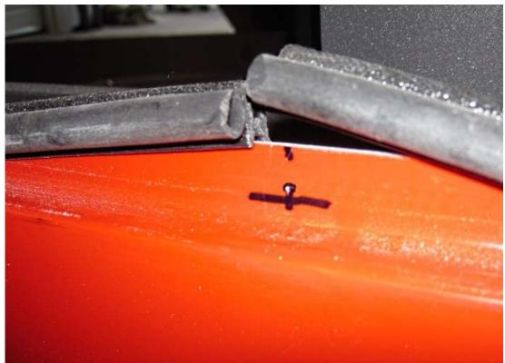
With the pin location compared to the trunk edge known and the trunk edge marked on the body along with the lowest mount point of the pin cover marked, the locations should match up. The latch cover may need to be trimmed slightly to go onto the radius of the body.
