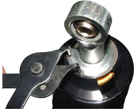
Install the snap ring on the spring hat so that it holds onto the shock end. Make sure that the slot in the snap ring and the slot in the spring hat are not aligned.
