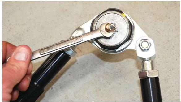
Screw the grease fittings in to the ball joints and tighten with a <sup>3</sup>/<sub>8</sub>" wrench.
