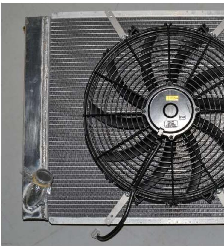
Place the fan on the radiator and rotate the mounts so that the smaller holes line up with the radiator flange.
