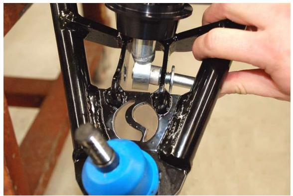
Pass the shock assembly (with the body of the shock up) through the upper A-arm and attach them to the lower control arm using the 0.43" spacers that are supplied in the kit.
