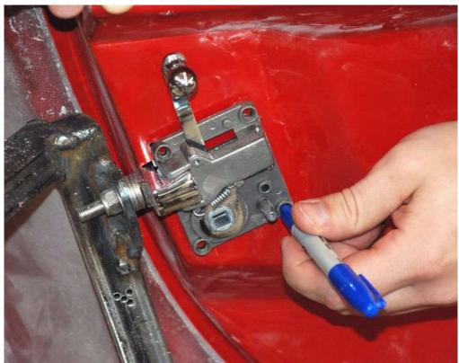
With the door lined up and the striker in place, mark and drill the 1/8" holes for the door latch.
