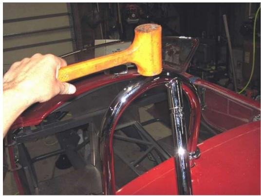
If necessary, use a plastic mallet to seat the rollbar hoop down and make sure the rear leg goes all the way up onto the hoop.
