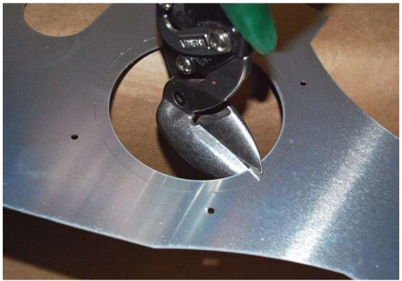
Depending on which gauges you are using you may need to open up the dash holes for the tachometer and speedometer. If you need the larger holes the take a tin snip and cut through from the smaller hole to the tracing for the larger one halfway between all the tabs.
