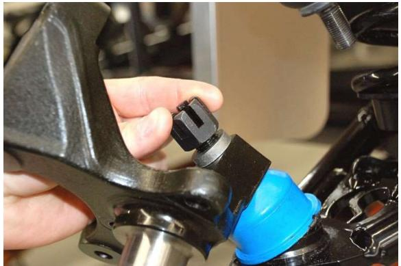
Place the spacer under the castle nut to ensure that the cotter pin is at the correct height. Torque to 108-122Nm (80-90 lb-ft) and install the cotter pin.
