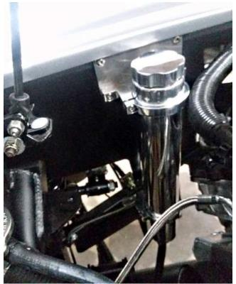
Pick the mounting location for the tank and mark the holes. Make sure the tank is accessible and visible inside to check the level on the finished car then bolt it in place.
