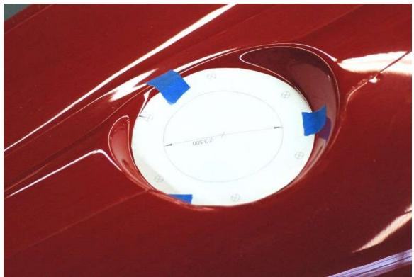
Locate the template in the appendix and only cut out around the outside diameter of the circle. Tape the circle in the gas cap recess of the body.
