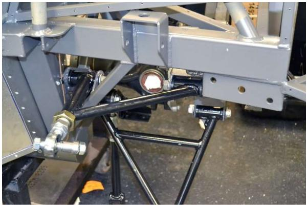
Pass the upper control arm thick tube through the triangular area as shown in between the frame mounts. Use the longer M16 x 110mm ( $\sim 4^{5}/_{16}$ ") bolts.
