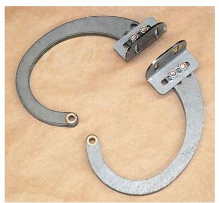
Use the carriage bolts and  $\frac{5}{16}$  locknuts to bolt the mounting pads to the arms leaving them just snug so they can be moved without loosening the bolts.
