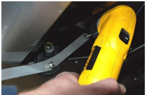
Using the inner hole of the bracket as a guide, drill the 2"x 2" outrigger all the way through both of the tube walls and into the footbox area with a  $\frac{5}{16}$ " bit.
