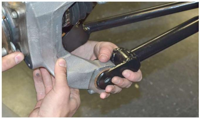
Attach the Toe link arm to the spindle using the M14 x 80mm bolt and locknut.
