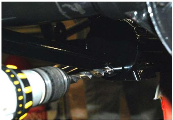
For the front mount, use a  $\frac{1}{2}$  drill bit and drill through the sleeve on the mount. Make sure before drilling that the hole is away from the side of the 2"x 3" tube so that a nut can be attached on the back of the bolt from the bottom of the tube.
