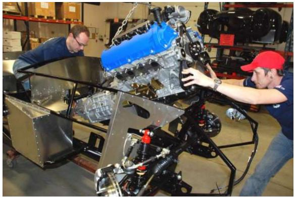
Lower the engine and transmission into place. The more hands you have to help the better. Go very slowly and make sure the transmission tail-shaft is above the rear cross-member.
