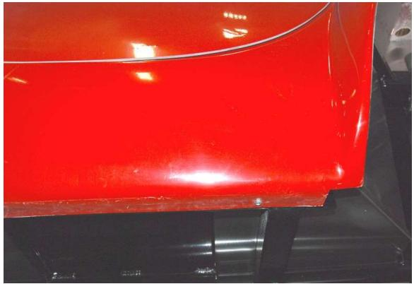
Unbolt the body sides from the chassis on the underside of the car.
