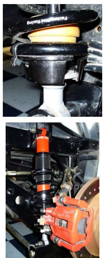
Run zip ties through the holes in the spring hat and around the spring to prevent the spring from becoming unseated.
