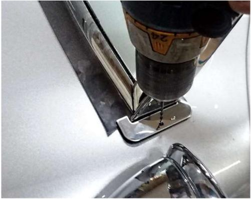
Use a 3/32" drill bit through the base plate holes for the mounting screws.
