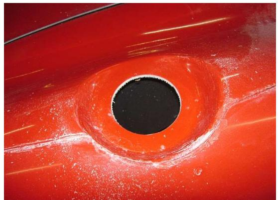
Use a  $3\frac{1}{2}$ " hole saw for the center opening. If you do not have a hole saw this size, you can cut the center circle out of the template and use the remaining template to mark for a jig-saw instead.
