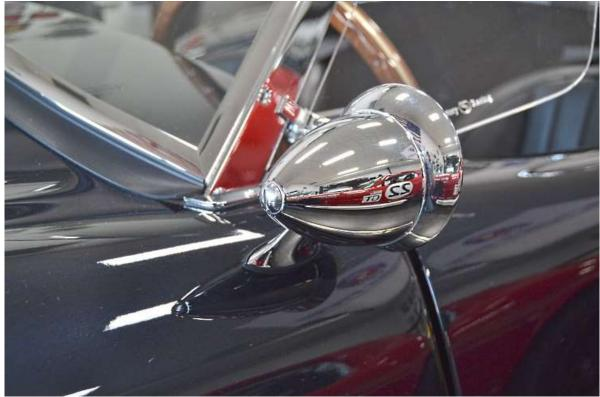
From the underside of the body, use a  $\frac{5}{16}$  socket to attach the mirror to the body.
