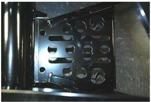
Jack the transmission up and mount the a-frame underneath it. Normally this mounts above the frame tabs but can be mounted underneath if extra clearance is needed.
