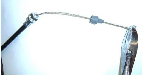
Cut the barrel fitting off the end of the cable.
