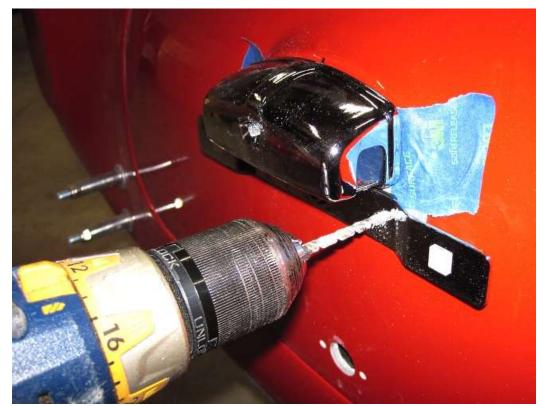
Push the light into the trunk and drill through the license plate mounting holes with a 3/16 drill bit.
