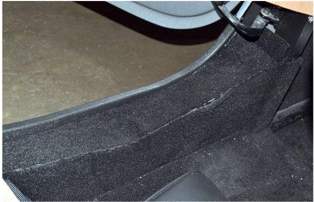
Install the under door top piece along with the push on weatherstrip.
