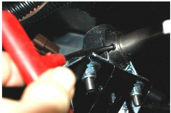
Tighten the set screws on the bearings using an <sup>1</sup>/<sub>8</sub>" Hex key.
