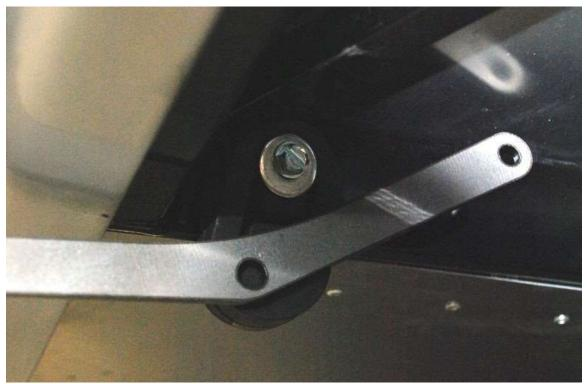
Screw the rubber hanger onto the chassis with the sheet metal mounting screw using one of the washers between the rubber and the head of the screw.
