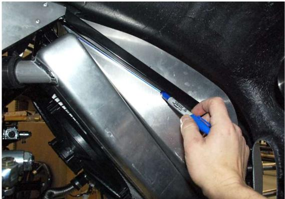
From the backside of the panel, mark the location of the  $\frac{3}{4}$ " tube.
