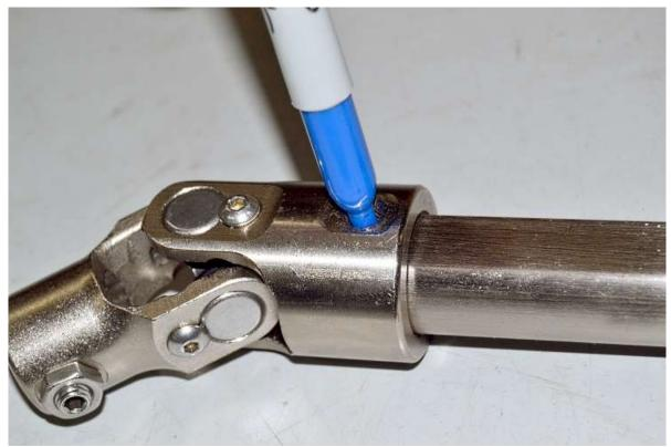
Mark the 1"DD tube through the set screw hole then remove the tube.
