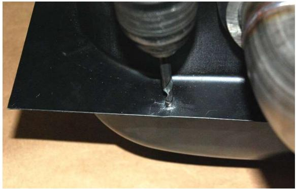
Drill a  $\frac{1}{4}$ " hole through the tank flange on the mark made.
