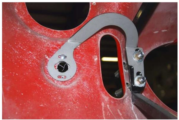
The body mounting bracket goes on the back side of the frame front mount.
