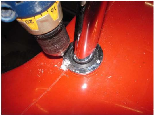
Locate and drill the front grommet holes.
