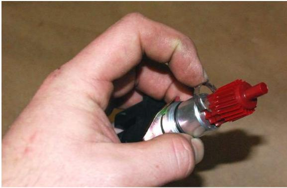
Install the gear on the end of the sender and hold it in place with the clip.
