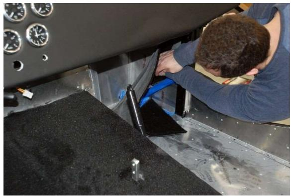
Fit and glue the right outside footbox wall carpet section. The carpet tucks in behind the footbox protection tube. Taping off the tube helps prevent getting the adhesive on it.
