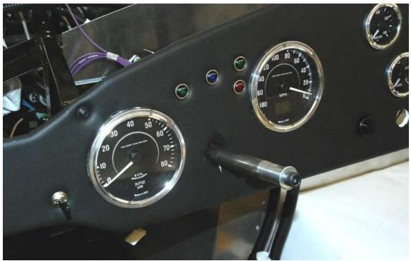
Mount the turn signal switch and high low beam switch as well as indicators in the dash. These can be mounted wherever you like, use a  $\frac{1}{2}$ " drill bit for the holes on both the switches and indicator lights.
