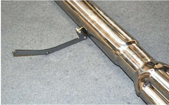
Bolt the mounting bracket to the pipe on the forward side of the bracket.
