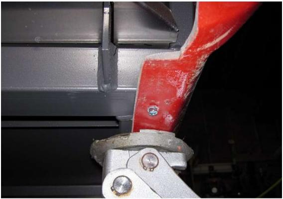
Once the front of the door is good, reuse one of the #10 self-tapping screws that the body was originally mounted with to lock the location in. Screw it up into the 2"x 2" tube near the front of the door.
