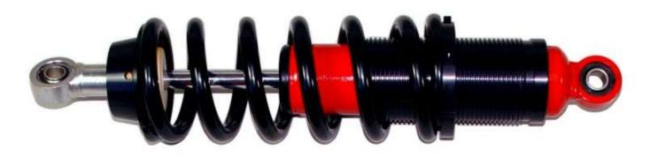
Put the spring and hat on the shock and rotate the spring seat back up the sleeve so that the spring pushes the hat tight against the end of the shock.
