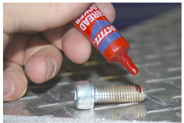
If the Hub was removed, use Loctite on the threads and reattach to the spindle.
