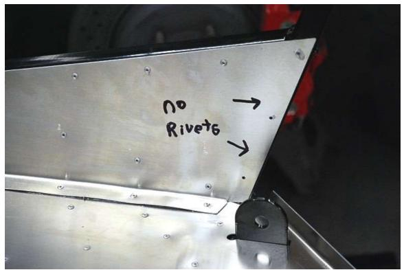
Drill, silicone, and rivet the right side under door piece in place. Leave the rivets out of the rear vertical flange for now.
