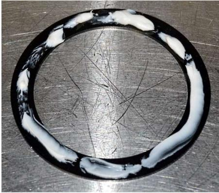
Place a small amount of white lithium or chassis grease on one side of the Delrin washer.
