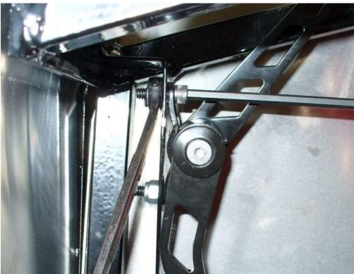
Bolt the pedal to the mount plate using the  $\frac{1}{4}$  x  $\frac{3}{4}$  screws and locknuts
