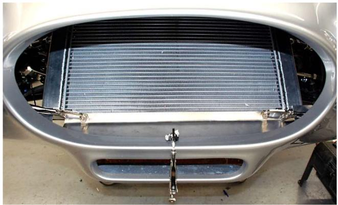
Attach the radiator floor piece to the bottom of the radiator with a couple of self-tapping screws on the marks or use a couple of clamps.
