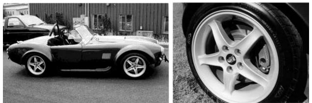
Left: FFR car using late model 17" Cobra-R rims. Right: Ford Racing Cobra R 17" wheels and 12" Cobra Brakes.
