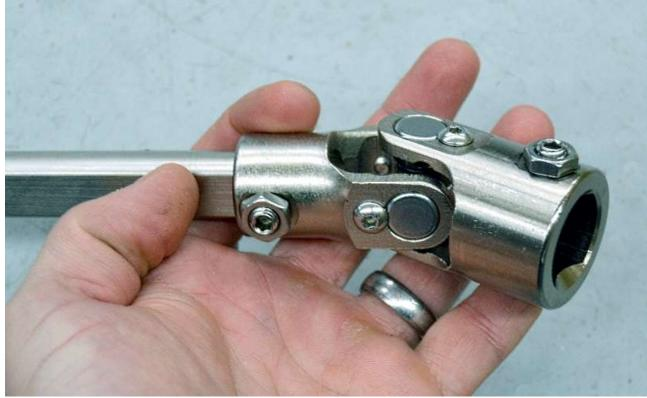
Push the  $\frac{3}{4}$ "DD end of the u-joint onto the  $\frac{3}{4}$ "DD shaft.
