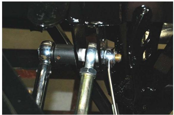
Jack the rear axle up and attach the upper link to the frame.
