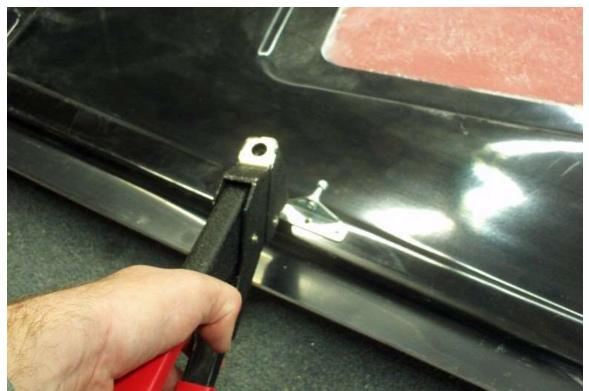
Install the ball pivots for the hood struts on the hood using 3/16" rivets. The ball points toward the inside of the car.
