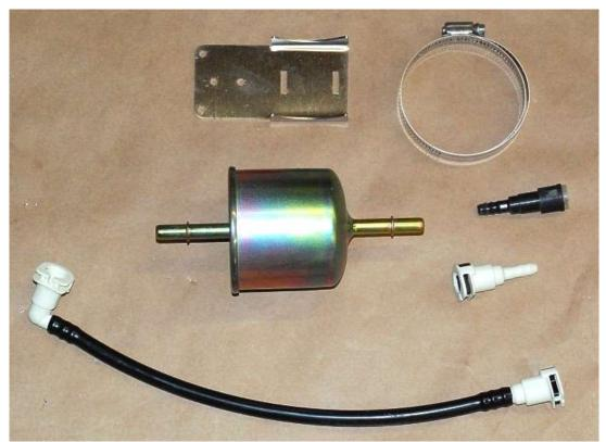
Unpack the fuel filter and mounting hardware.
