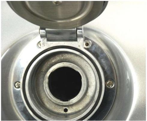
Set the cap on the body and screw in using 5 of the countersunk screws. Leave the inside most forward hole open.
