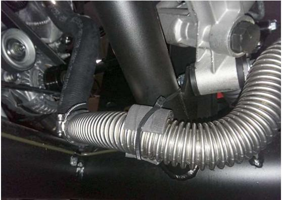
Where the tube goes under the X use one of the extra adapters and some kit zip ties to hold it against the X to prevent any shaking while driving.
