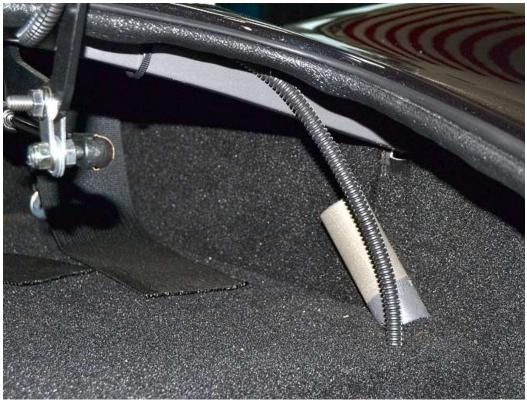
Pull the license plate wires up next to the right side rear rollbar leg.
