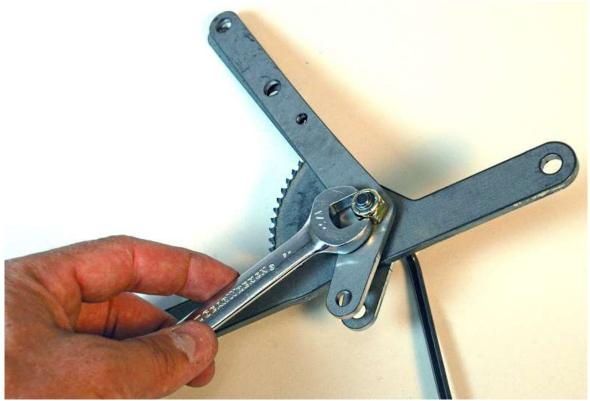
Using a  ${}^{3}/{}_{16}$ " hex key and  ${}^{1}/{}_{2}$ " wrench, tighten the shoulder bolt lock nut so that the ratchet to handle mount plates are against the bushings but they can still move up and down. Make sure the ratchet to handle mount plate next to the locknut does not get caught on the edge of the shoulder bolt.
