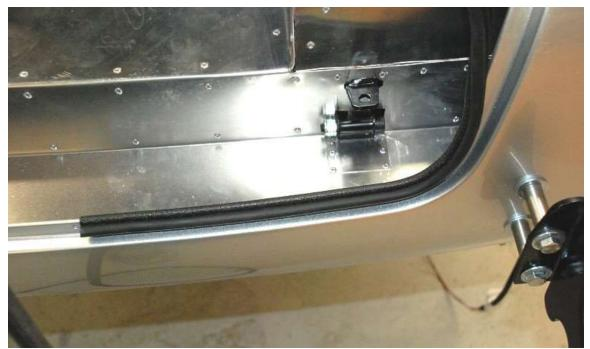
Push the side mount weatherstrip on the trunk opening starting at the bottom next to the latch pin hole and working all the way around just leaving a small gap for the head of the latch pin bolt.
