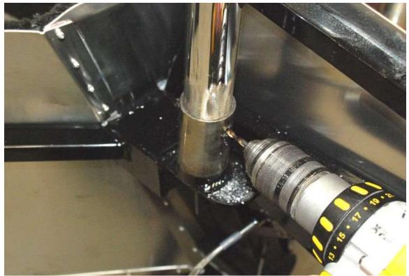
Drill a hole all the way through each of the lower mounts and rollbar main hoop.
