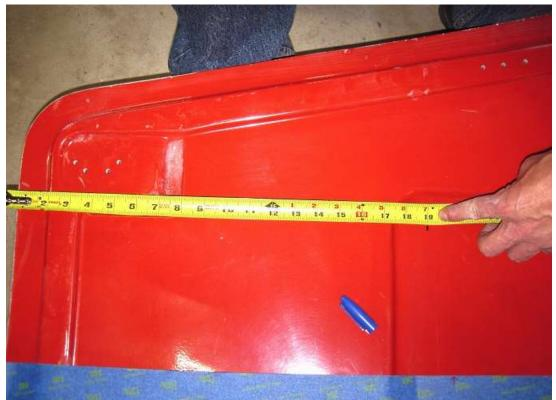
From the front edge of the hood measure back 19" and mark the underside of the hood.
