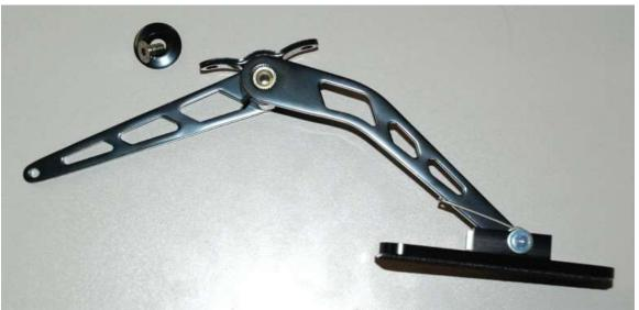
Unpack the throttle pedal and separate the arms. You can leave the screw loose for now as this will be adjusted for fit later.
