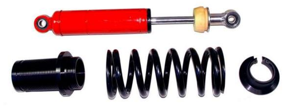
Unpack the shocks, coil-over's and hardware.
