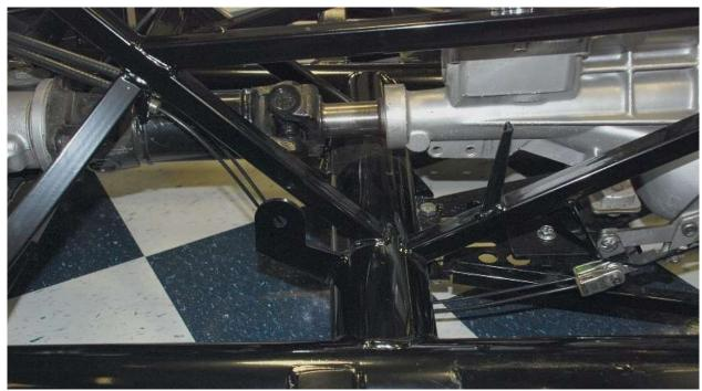
For 87-92 and FFR cables route the inner cable down under the chassis 4" crossmember.
