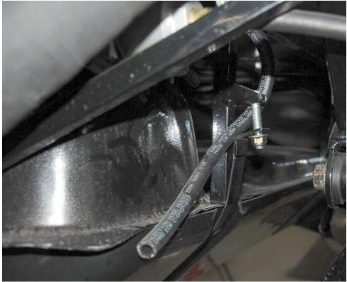
Run the vent hose down to the  $\frac{3}{4}$ " tube near the battery and attach it to the tube using a zip tie.
