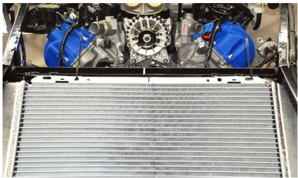
Mark the center of the radiator and the center of the chassis and offset the radiator by 5%".
