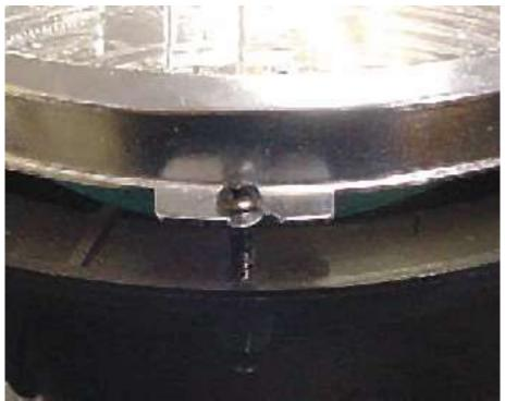
Plug the light into the connector and mount the bulb to the bucket. The slotted parts of the mounting flange go onto the adjusting screws between the screw head and flange.
