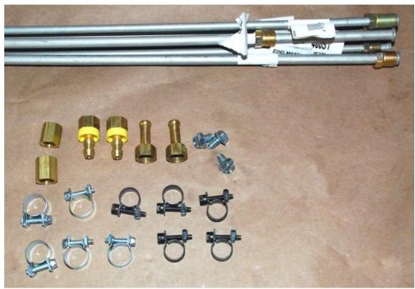
Unpack the fuel lines and the fuel line assembly which is in the secondary chassis components box.
