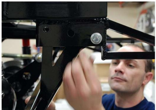
With the axle jacked up, attach the Panhard Bar frame mount to the inside of the quad shock brackets, the forward leg will attach to the back of the angled 2"x 3" tube. Do not tighten the quad shock bracket bolts yet.
