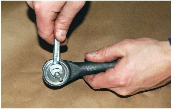
Screw the grease nipple into the outer tie rod end.
