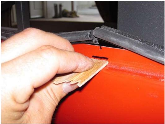
Use a paint stick or what was used to set the gap of the trunk to draw a line on the body where the edge of the trunk will be.
