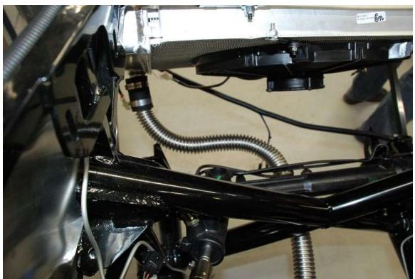
Make sure that the lower hose is not hanging down. If necessary, zip tie the hose to the frame.
