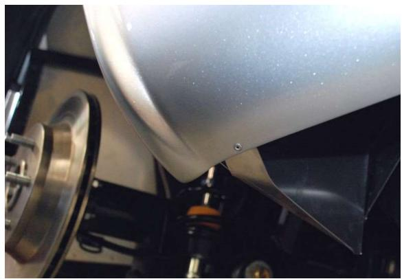
Use a long  $\frac{1}{8}$ " rivet as low as possible to attach the tab to the lower fender.
