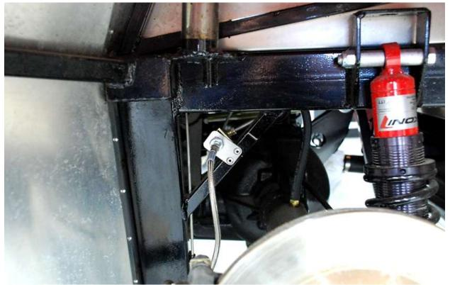
Using the FFR rear brakes, we attached the flexible brake line mount to the driver side diagonal <sup>3</sup>/<sub>4</sub>" tube with the brake line clip.
