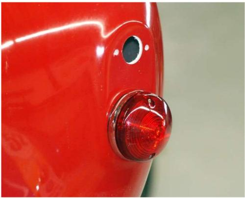
Test fit the lights and file the holes to fit if needed.
