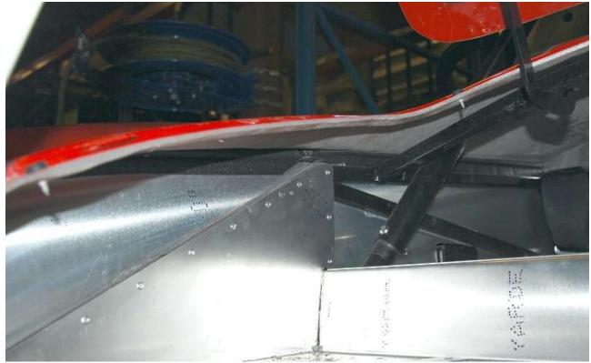
The push-on weather strip goes across the top of the trunk walls and rear floor.
