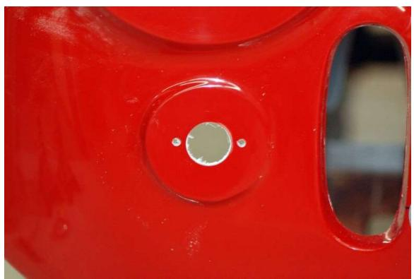
Drill the outer holes with a  $\frac{7}{32}$  drill bit and the inner with a  $1\frac{1}{4}$  hole saw.
