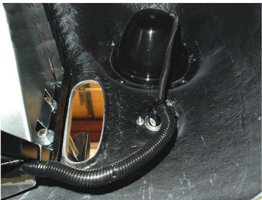
Wire in the headlights to the chassis harness. On the headlight, there are three wires, black is ground, white is high beam and the red is low beam.
