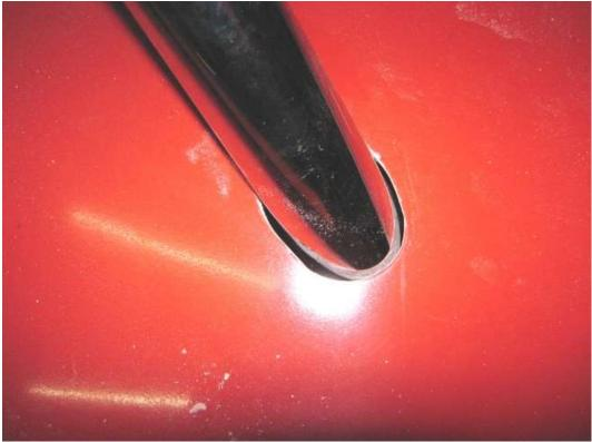
Trim the remaining flash on the opening with a file or jig saw.
