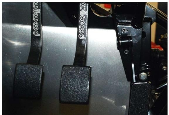
Use one  $\frac{1}{4}$  x  $\frac{3}{4}$  screw and locknut from the pedal box hardware position the accelerator pedal using the top hole in the accelerator pedal mount so that the top of the pedal lines up with the accelerator cable hole so the cable will come out straight. Mark the lower accelerator pedal mount hole then drill the plate to bolt the pedal in place.
