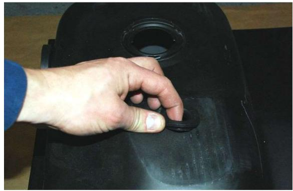
Insert the small rubber vent gasket in the small hole on the top of the tank.
